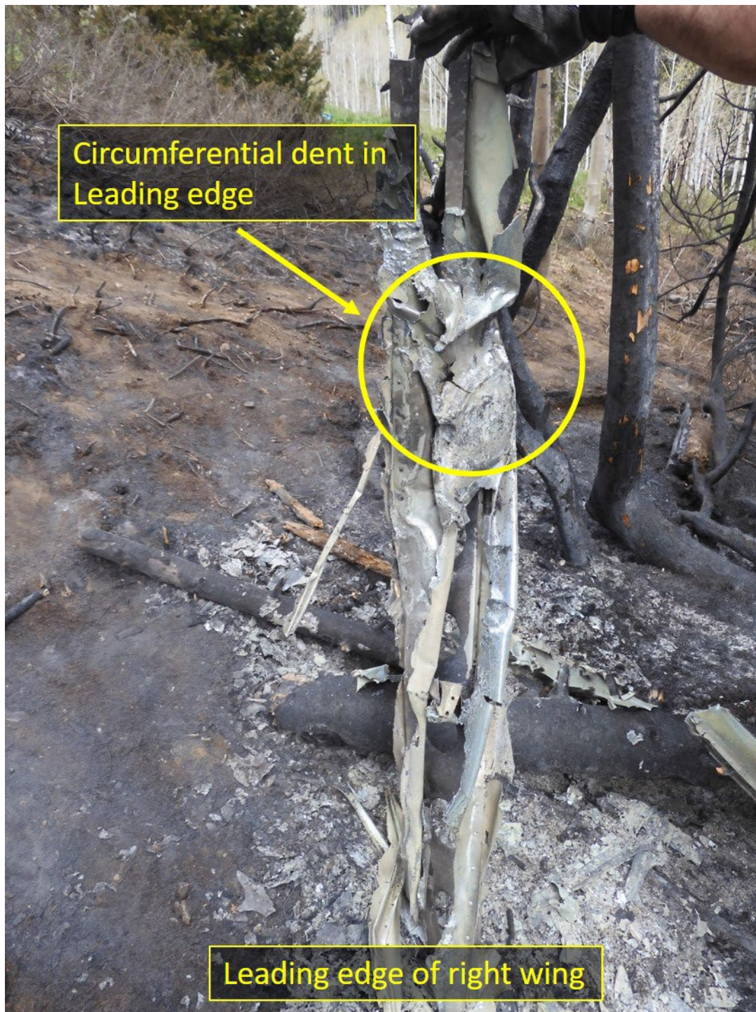
Figure 15. Remnant of the right-wing leading edge.
