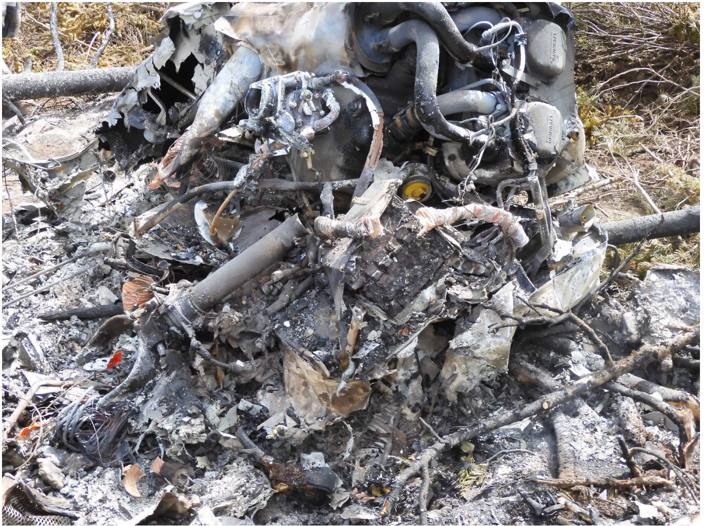
Figure 14. Underside of the engine showing the nose wheel strut.
