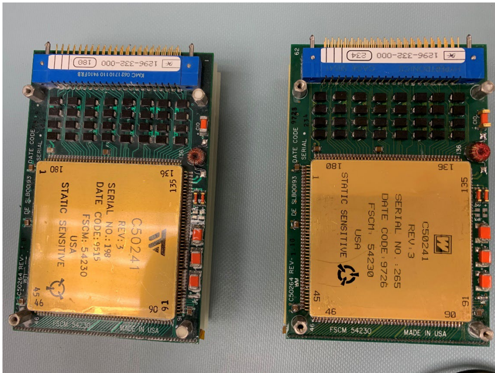
Figure 5. Memory modules swap: the known good memory is on the left and the accident memory is on the right.
