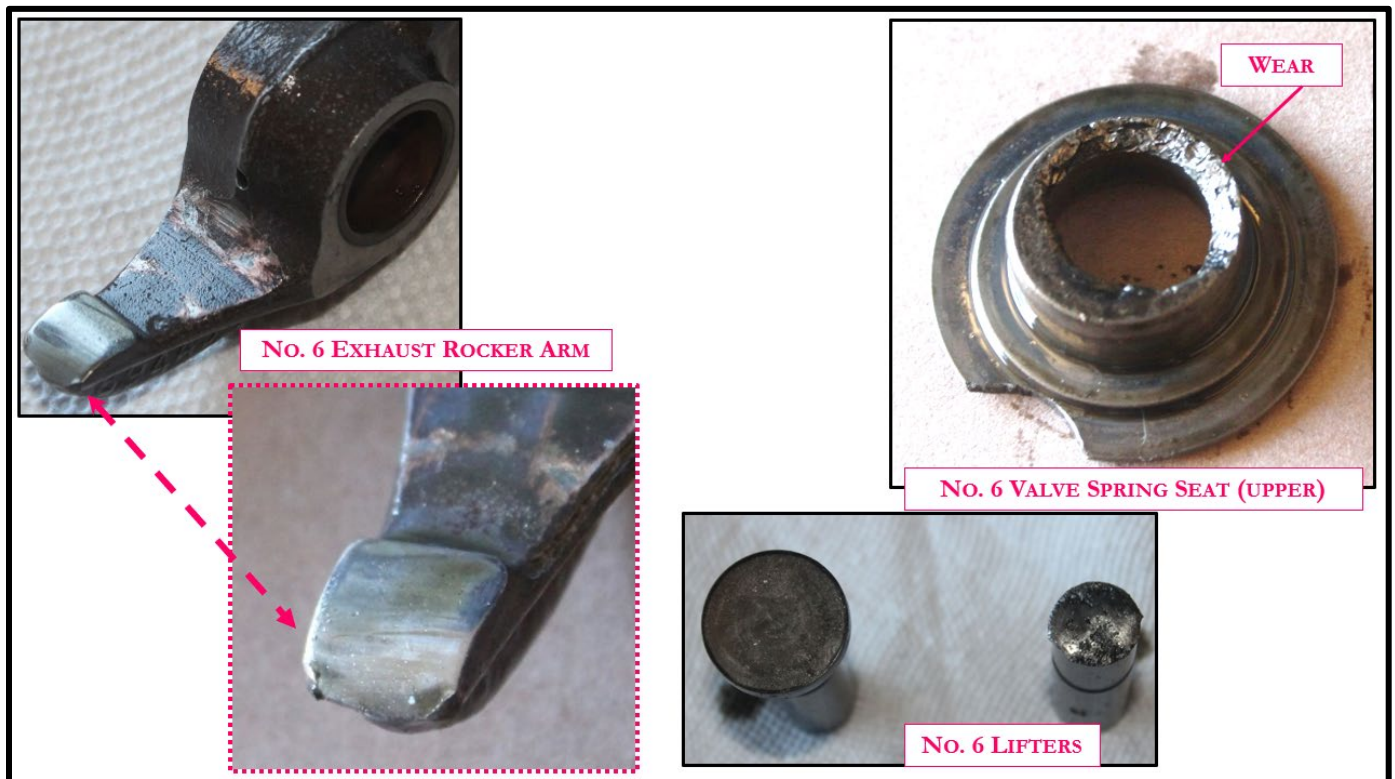
Figure 24: No. 6 Exhaust Cylinder Components
