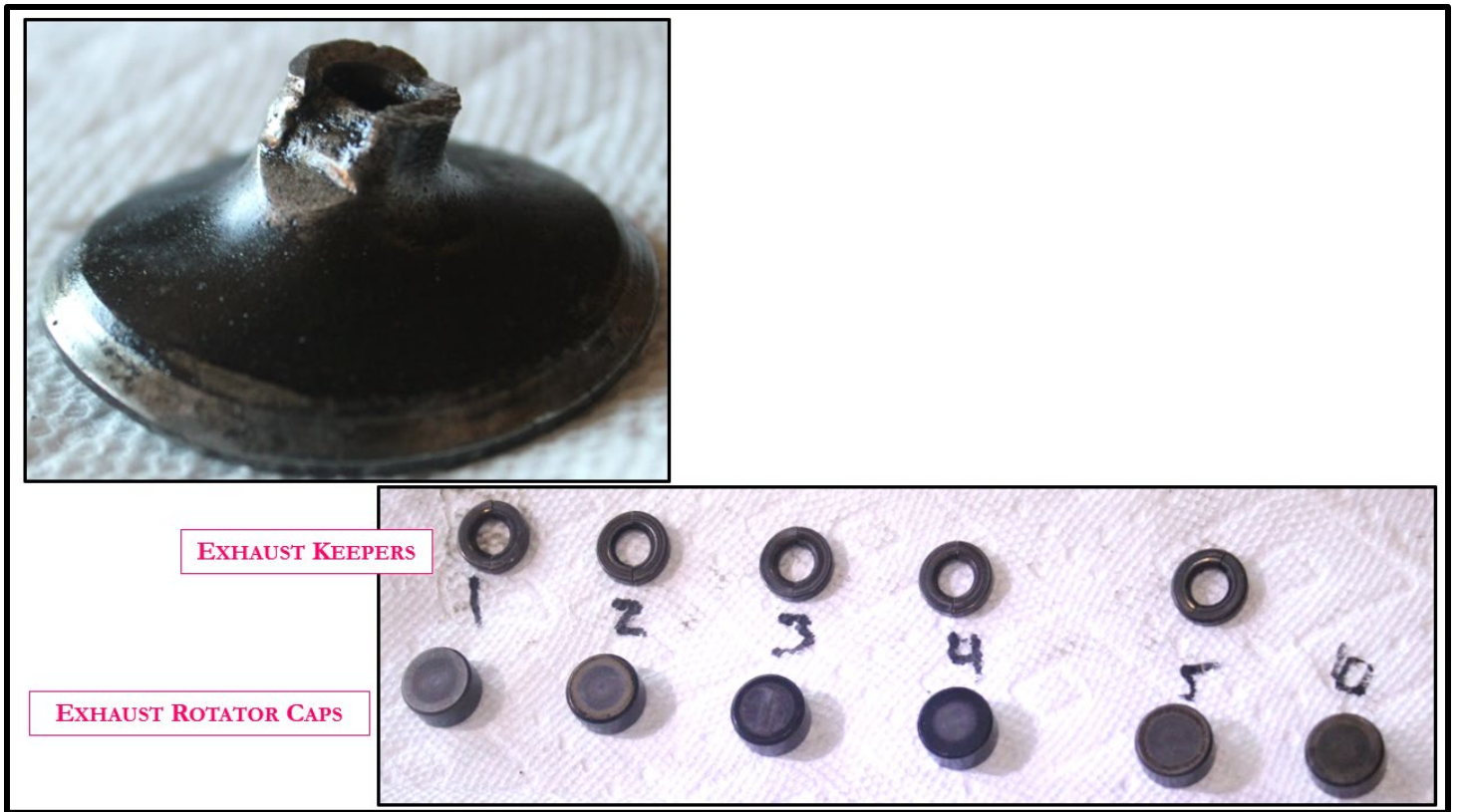
Figure 25: No. 6 Exhaust Valve Head and Comparison of Keepers and Rotator Caps
