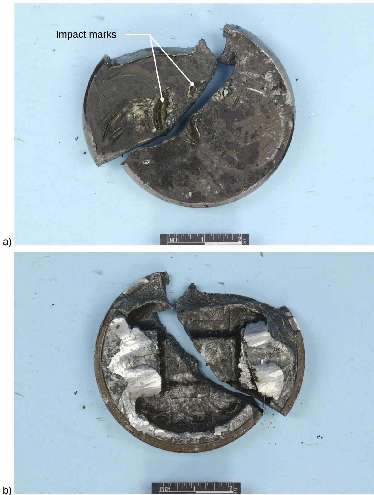
Figure 2: Images of fractured piston; a) piston-crown side and b) inward side showing fracture in-plane with the pin bosses.
