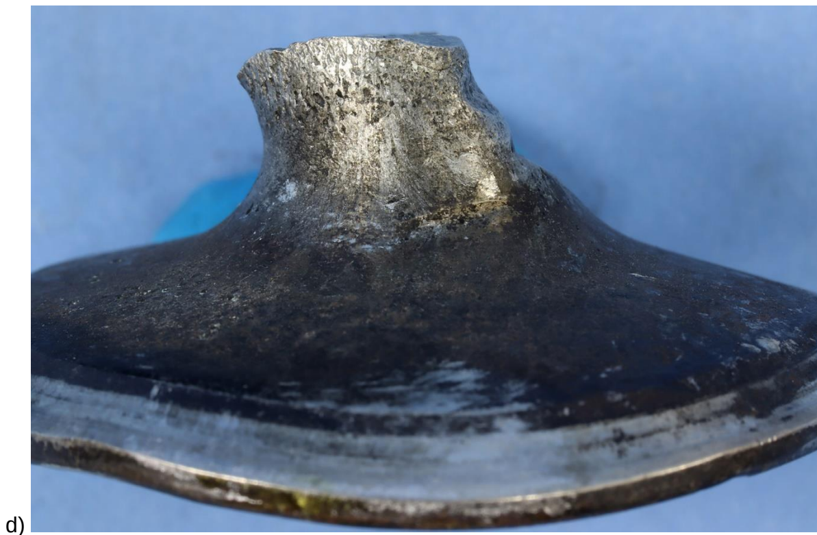
Figure 6 (cont.): c) higher magnification image of the stem fracture; d) side view showing shear deformation of stem adjacent to fracture; and
