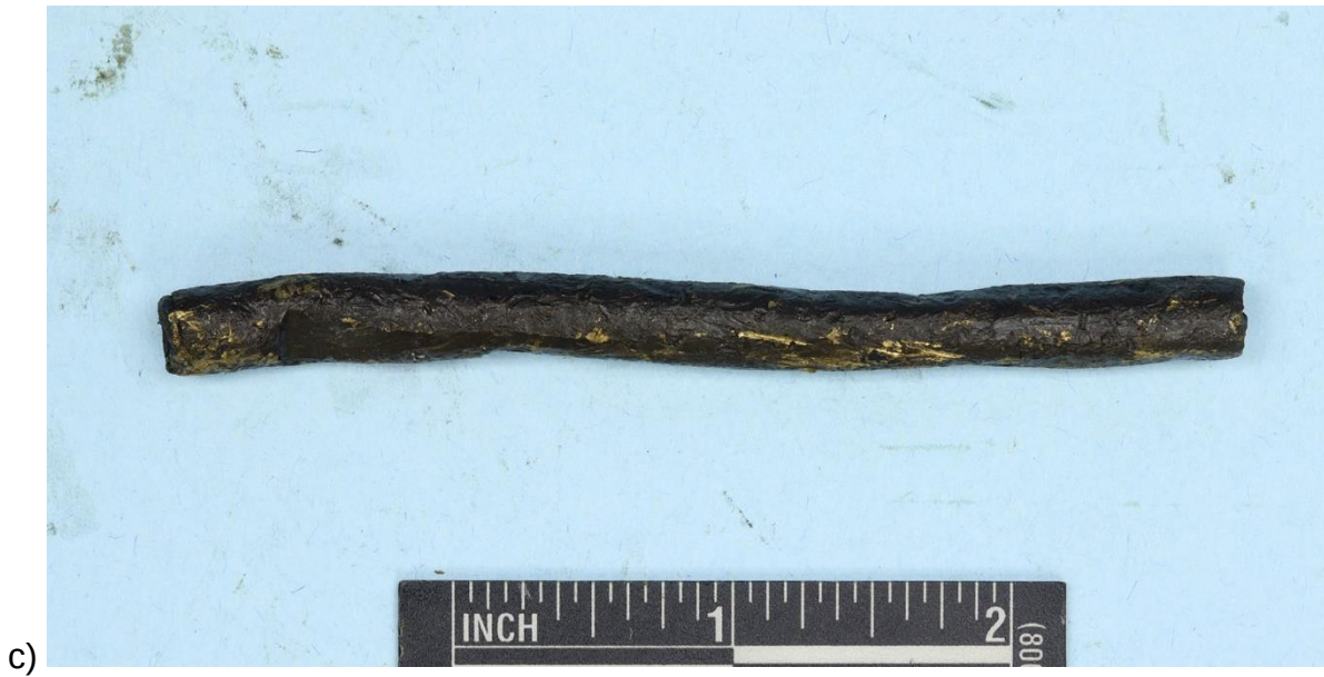
Figure 1 (cont.): c) piece of rod found in oil sump.
