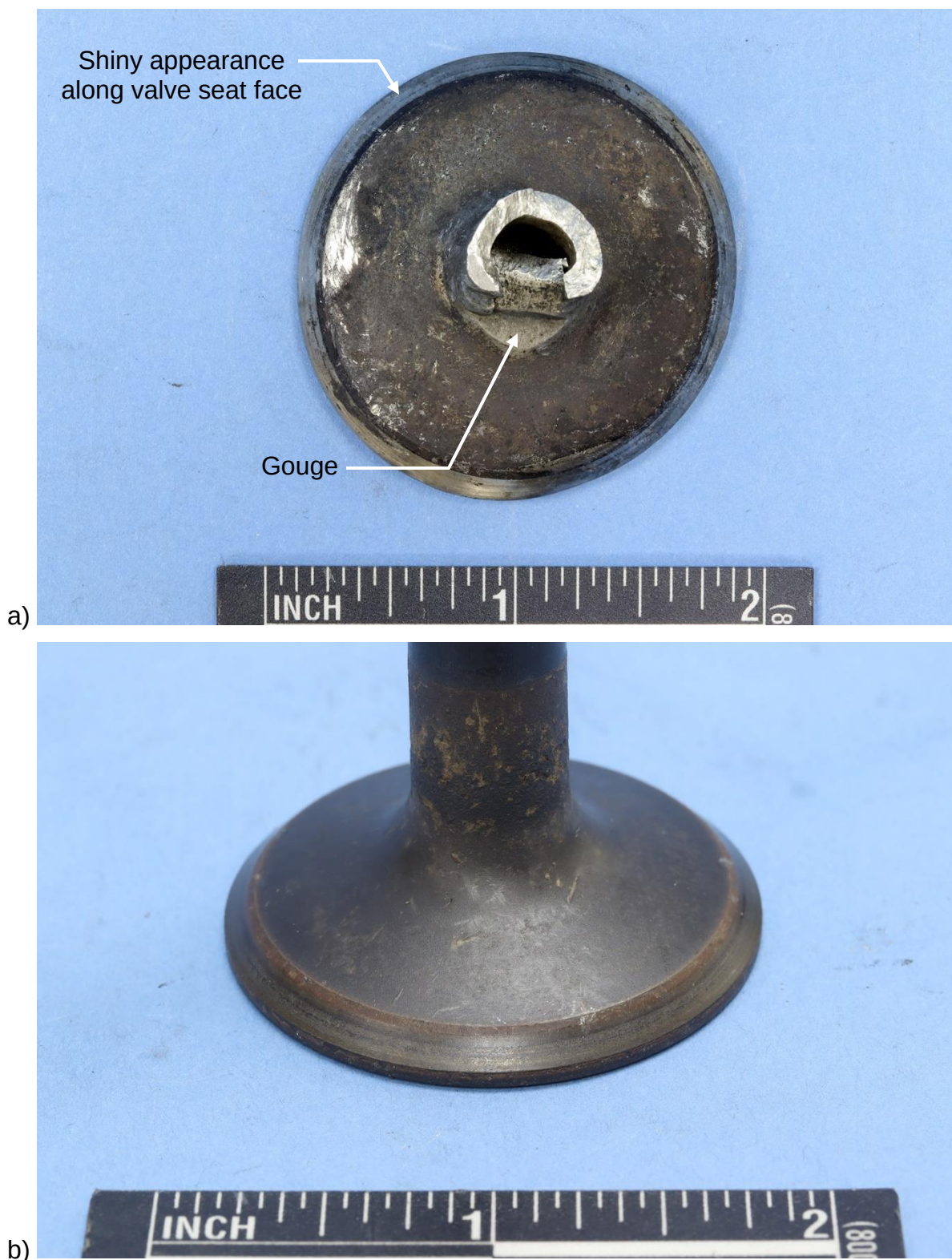
Figure 6: a) Image of the number 6 exhaust valve showing the fractured stem, outer face of the valve head and valve seat face; b) image of the number 5 exhaust valve;
