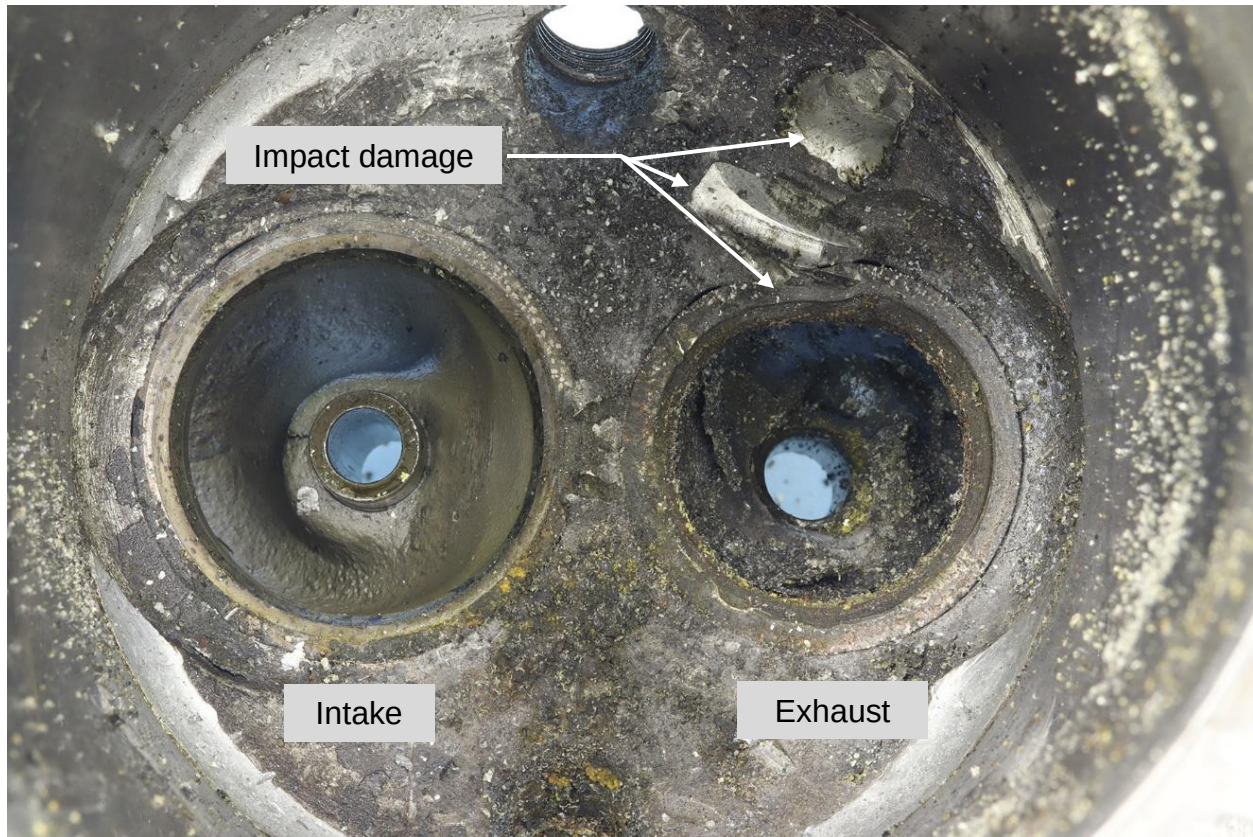
Figure 3: Inside view of number 6 cylinder head showing damage to the exhaust valve seat and surrounding material.
