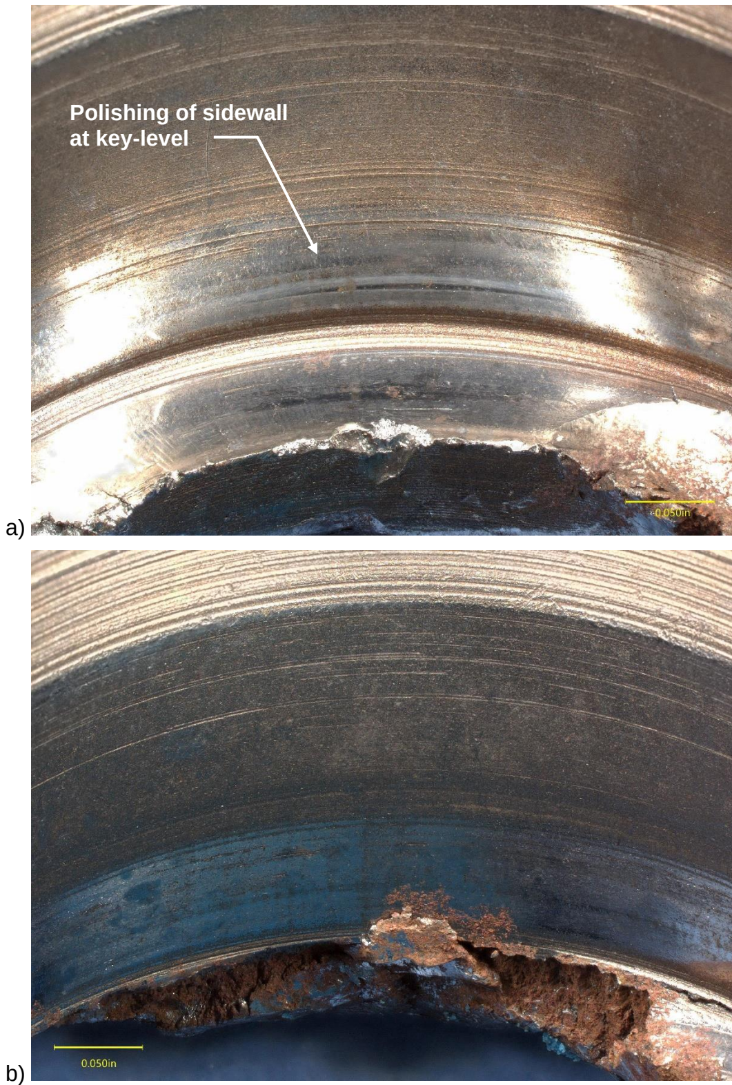
Figure 10: Images of the number 6 exhaust valve upper spring seat cup sidewall; a) 0°; b) 90°;
