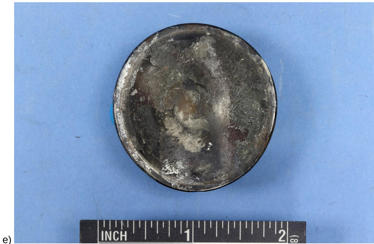
Figure 6 (cont.): e) image showing the combustion face of number 6 exhaust valve.
