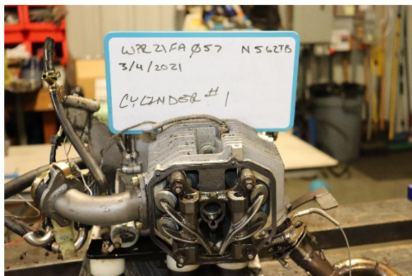
Figure 3. View of right cylinder rocker arm and valves
