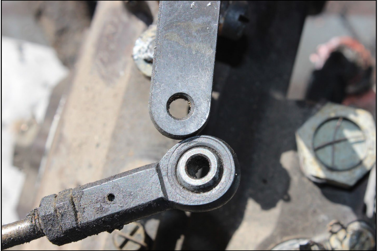
Figure 2: The throttle linkage control lever rod end and control arm with soot cleaned off.
