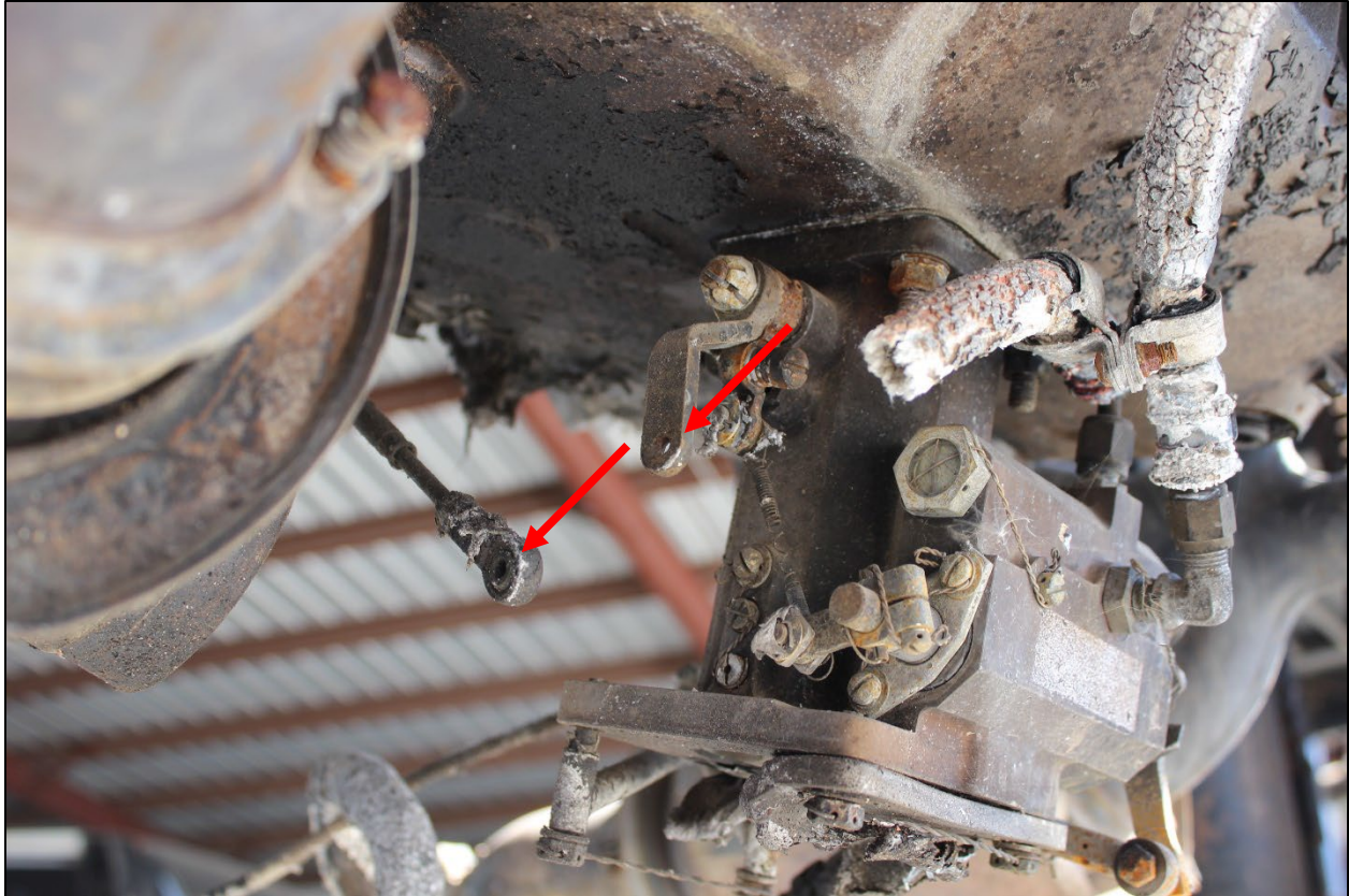
Figure 1: The throttle linkage control lever rod end disconnected to the control arm of the fuel servo.
