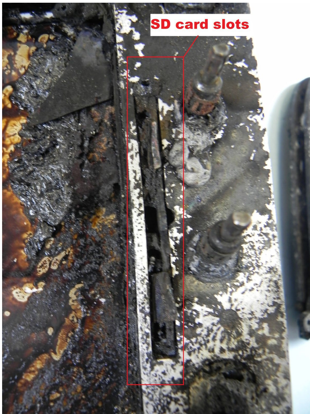
Figure 4. View of Garmin G1000 SD Card slots.
