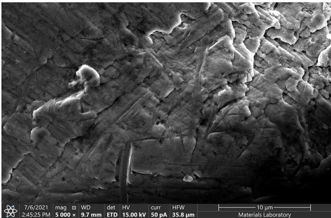
Figure 35 – SE micrograph of a closer view of the wear damage in Figure 34.
