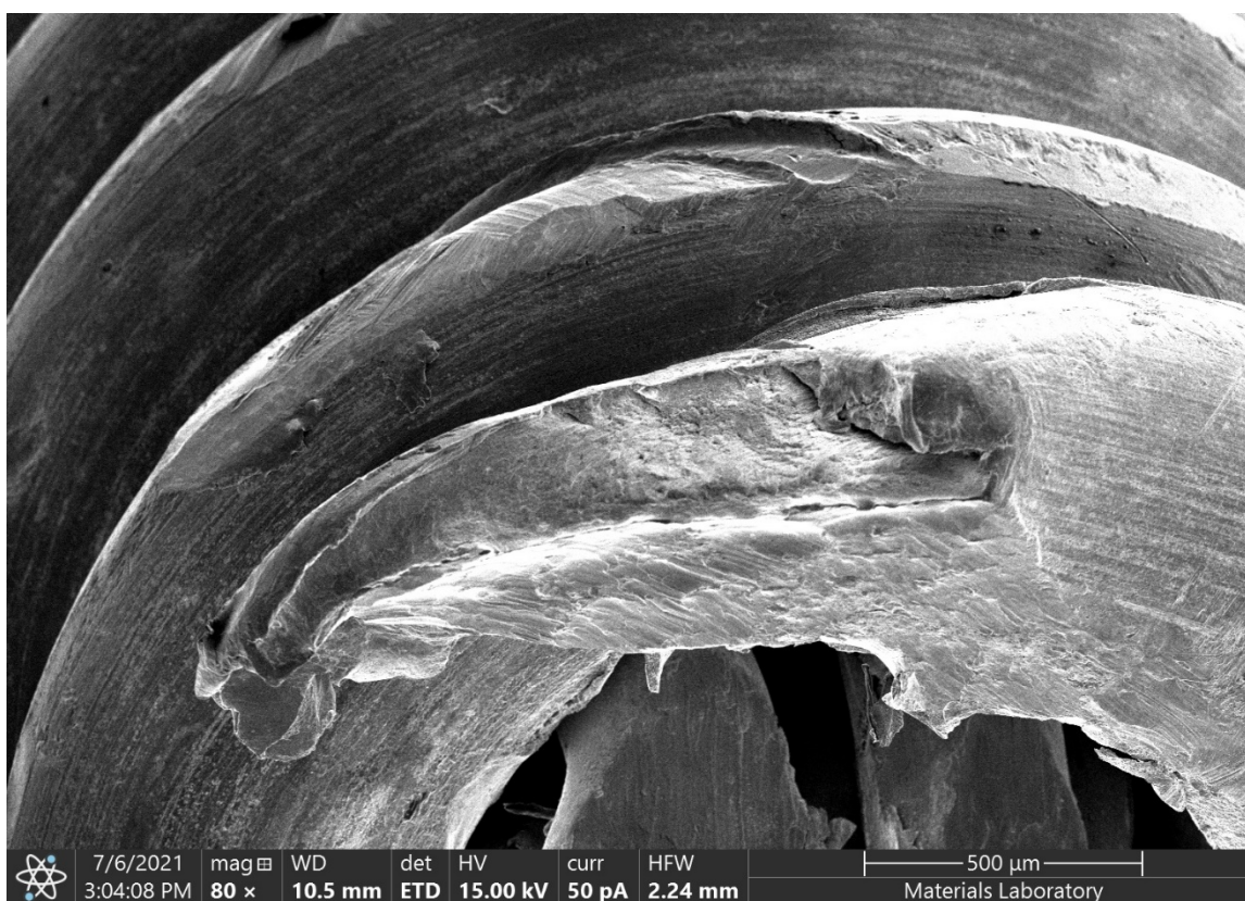
Figure 25 – SE micrograph of an angled view of the outer sheath coil fracture surface and wear damage along adjacent coils.
