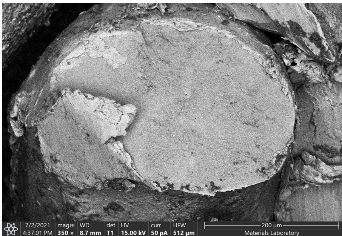
Figure 7 – Backscattered electron (BE) micrograph of the Strand 1 fracture surface.
