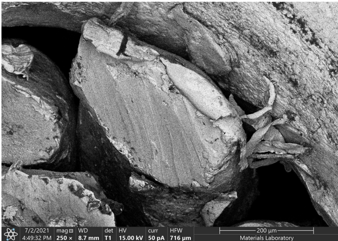
Figure 15 – BE micrograph of the Strand 3 fracture surface.
