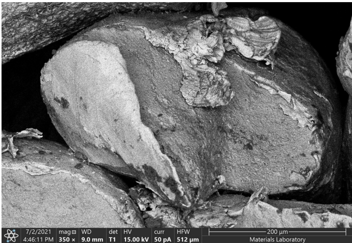
Figure 11 – BE micrograph of the Strand 2 fracture surface.
