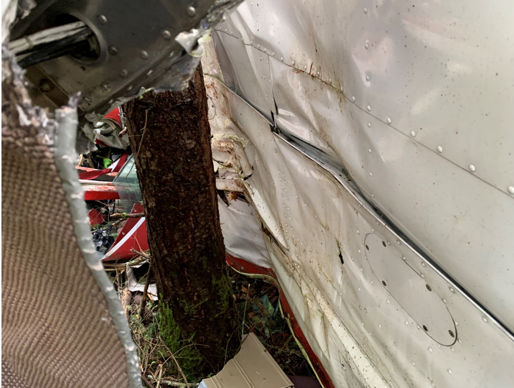
Figure 5: Right Wing Damage Consistent with Tree Impact.
