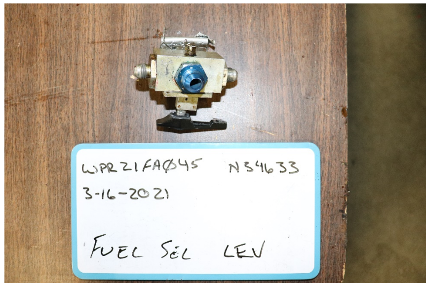
Figure 5: Fuel selector valve
