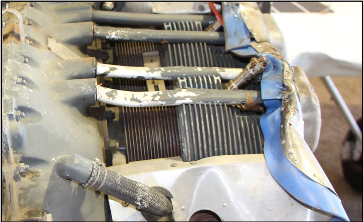
Photograph 4: Cylinder 2 Intake and Exhaust Push Rods
