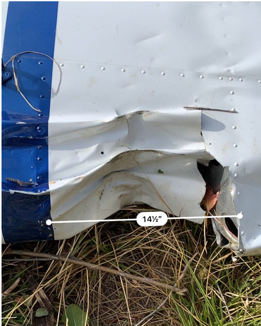
Photograph 2: Depression in right wing and tree remnants
