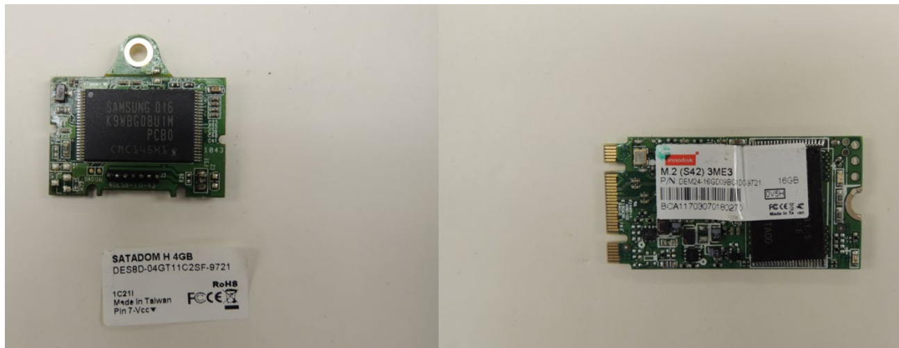
Figure 3: Memory modules from SV D700 (left) and SV HDX (right).
