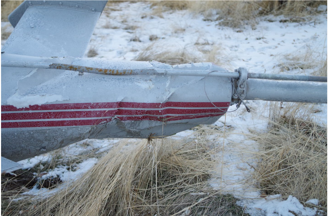
Figure 7. View of the damaged area of the tailboom bear the location of the tail rotor blades. Photo courtesy of the pilot.
