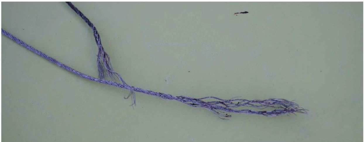
Figure 9. Left-side tail rotor control cable, showing the fracture. Photo courtesy of the airframe manufacturer.
