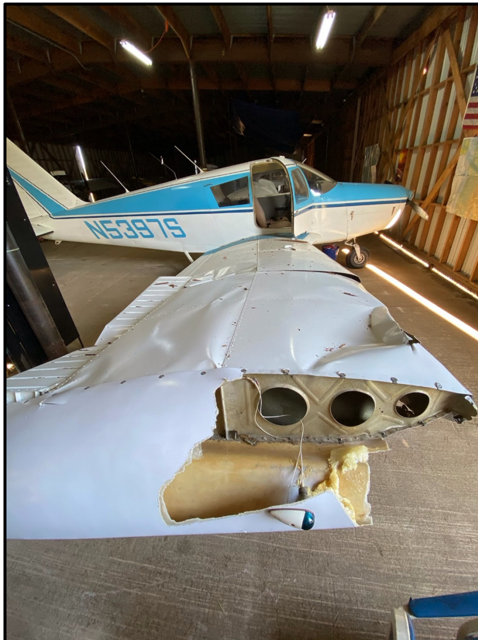
Figure 1: Airplane Right Wing Damage
