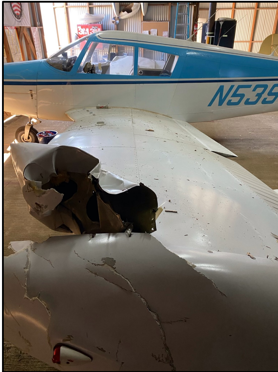
Figure 2: Airplane Left Wing Damage
