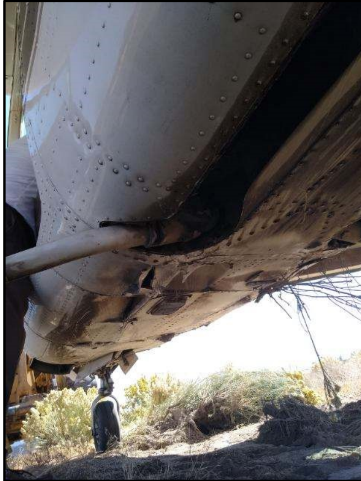
Figure 1: Airplane belly damage as viewed from the rear. (Courtesy of FAA).
