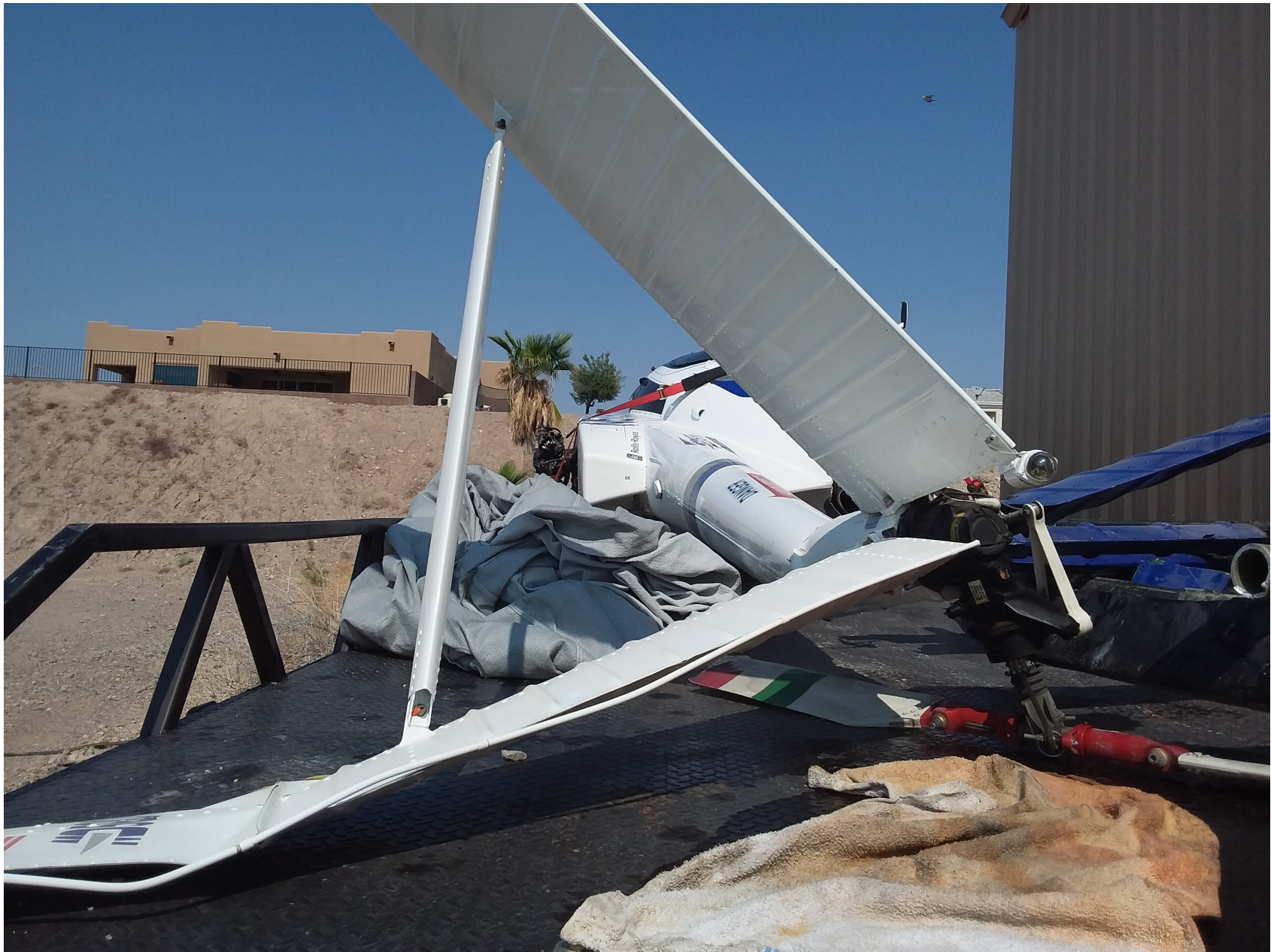
Photo 4 – N509CG, Rear view, showing damage to the tail boom. Photo courtesy of the pilot.
