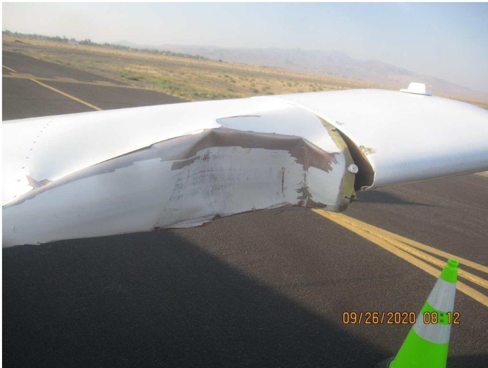
Photo 2 -N4132W, showing damage to the left-wing leading edge. Photo courtesy of the pilot.
