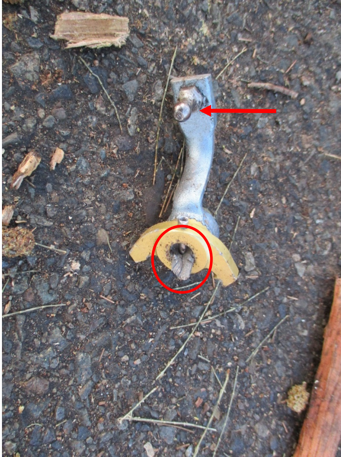
Figure 8 - Photo 8 of 11, N3617L Mixture Control Arm, courtesy of Airport Ops
