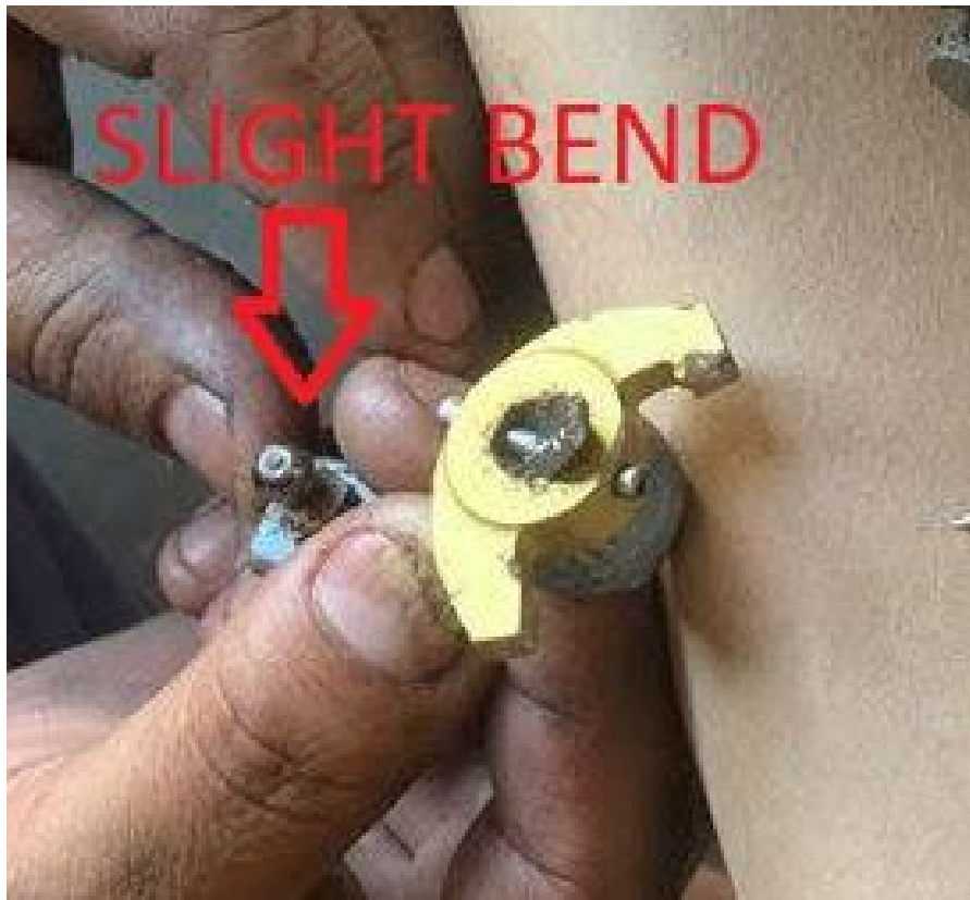
Figure 10 - Photo 10 of 11, N3617L Bent Ball Joint, courtesy of NTSB
