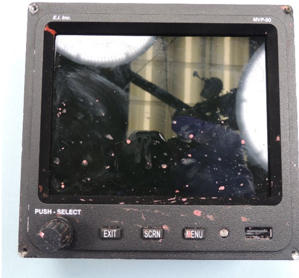
Figure 3: Electronics International MVP-50T as received.
