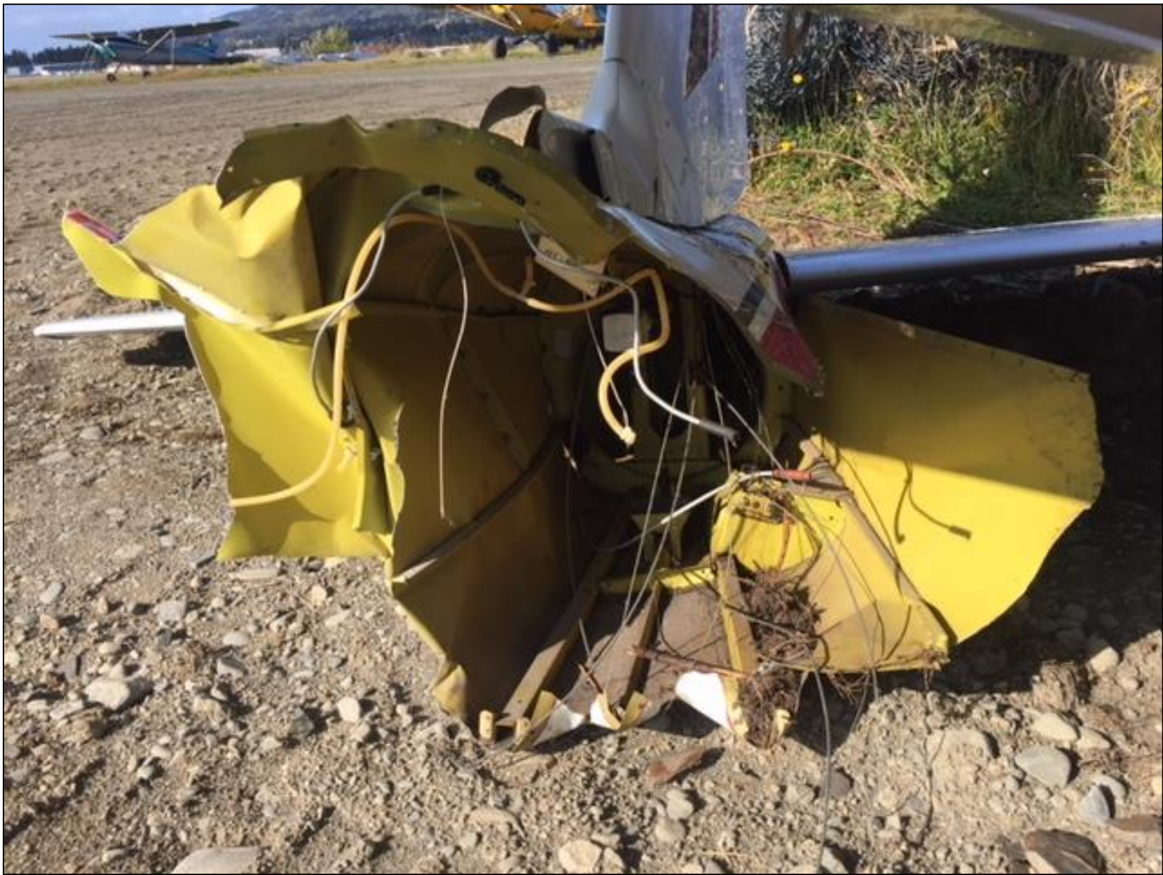
Photo 7 – Accident site, forward view of the separated empennage.
