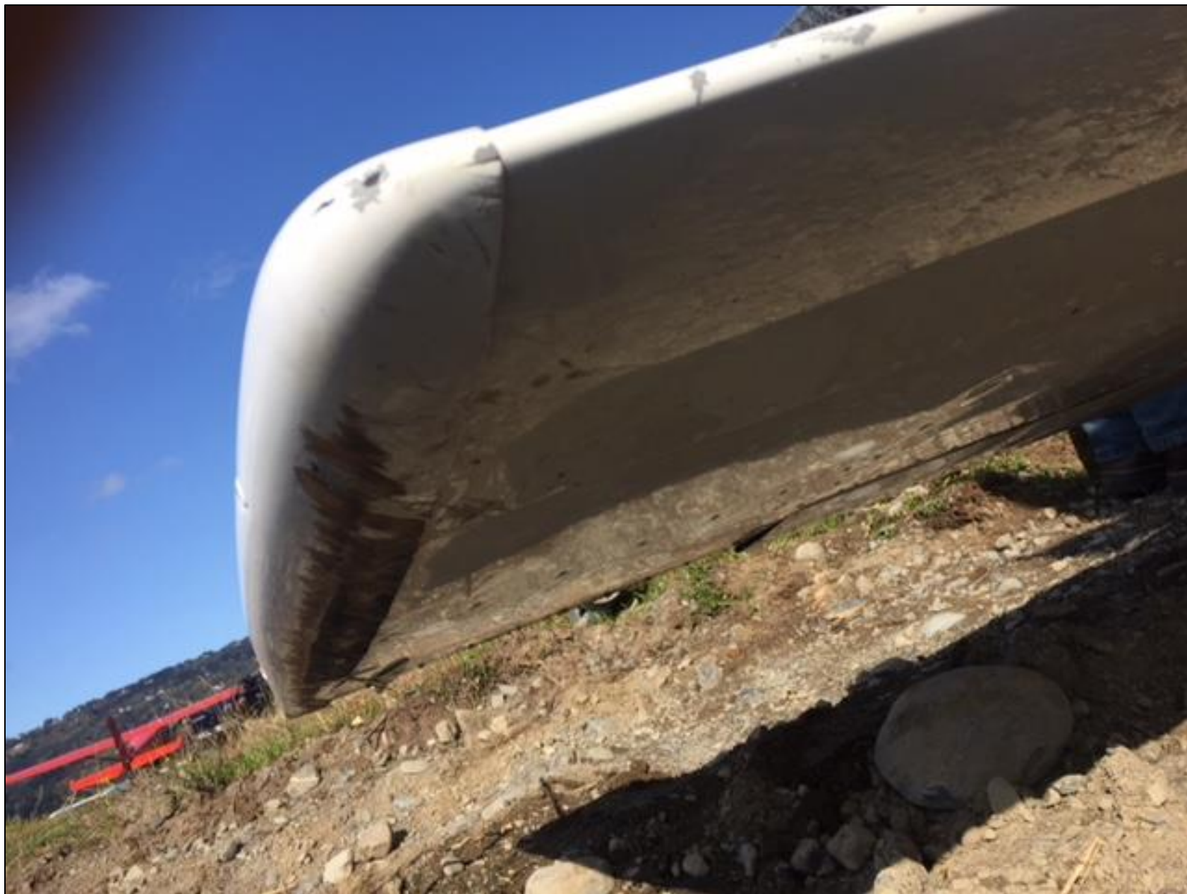
Photo 10 – Accident site, view of the right horizontal stabilizer tip.
