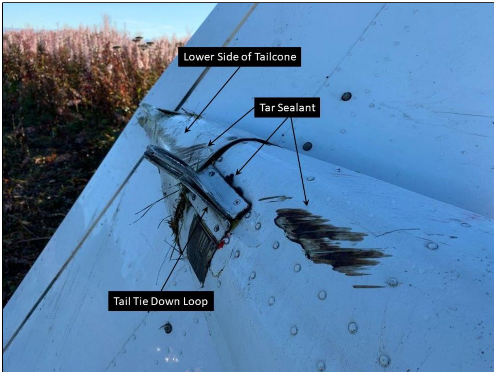
Photo 5 – Accident site, lower view of the tail cone and tail tie down loop.
