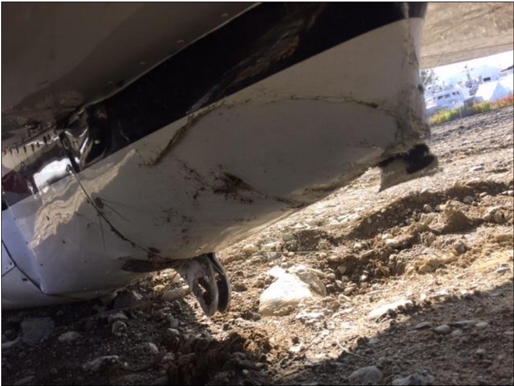
Photo 4 – Accident site, lower left side view of the tail cone and tie down loop.
