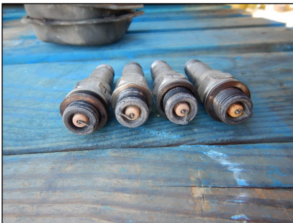
Figure 7-Right engine upper sparkplugs.
