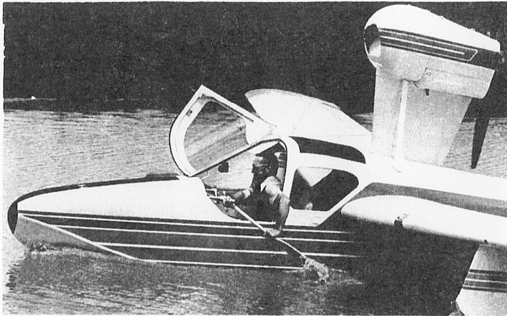
The LAKE may be paddled the last few feet to the dock or shore while maintaining direction control from the cockpit.
