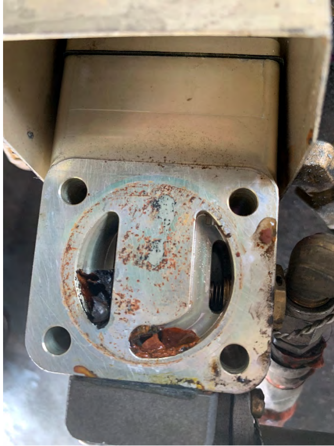
Figure 3: View of the fuel pump with corrosion and dirt like debris within the internal cavities.
