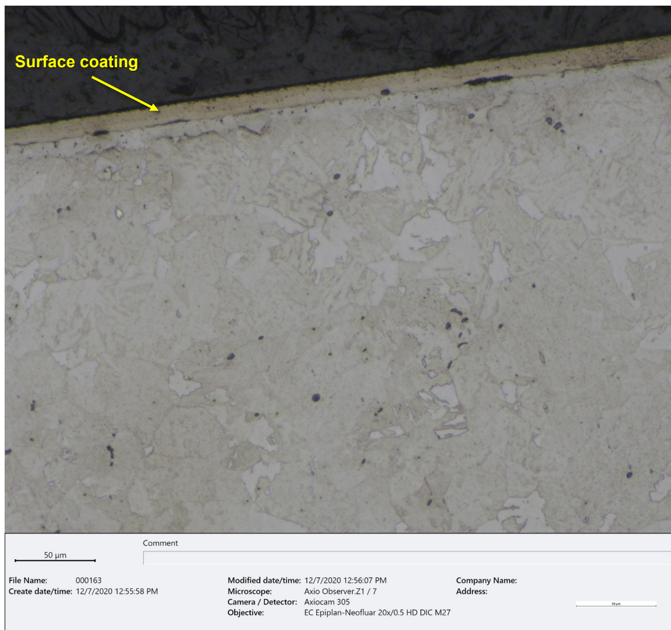
Figure 21 – Bright-field (BF) optical micrograph of a cross section of the collar surface, parallel to the fracture surface, showing the adherent surface coating (~200X, etched 2% Nital).
