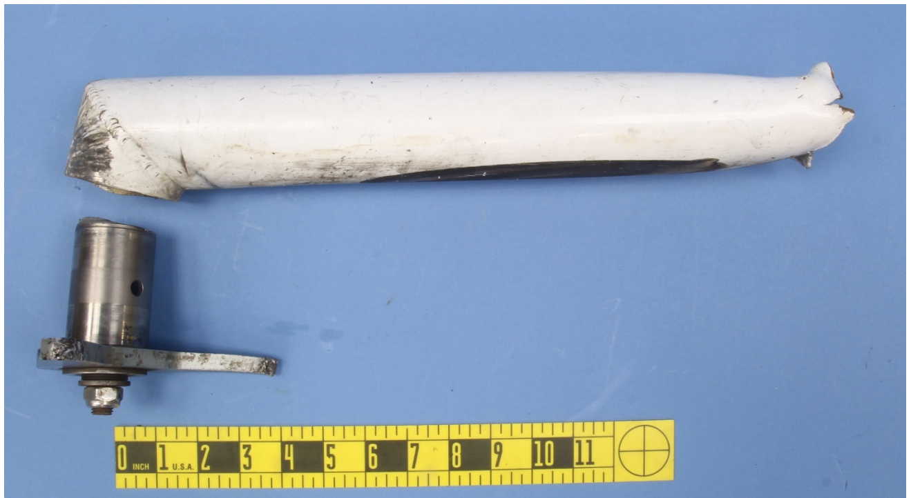
Figure 2 – Remnant of the NLG leg welding assembly, which fractured at the fork collar location. The stop plate was still attached to the leg collar remnant.
