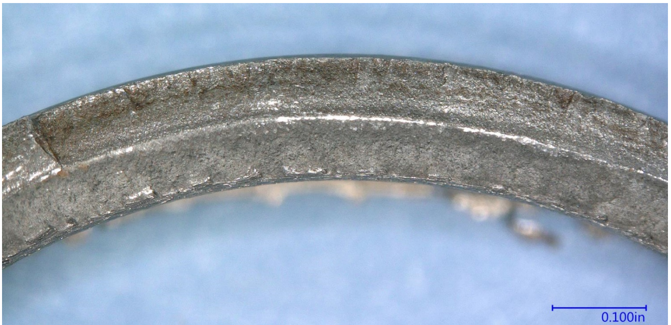
Figure 9 – View of the fatigue crack 2, showing the depth of fatigue crack penetration through the collar cross section.
