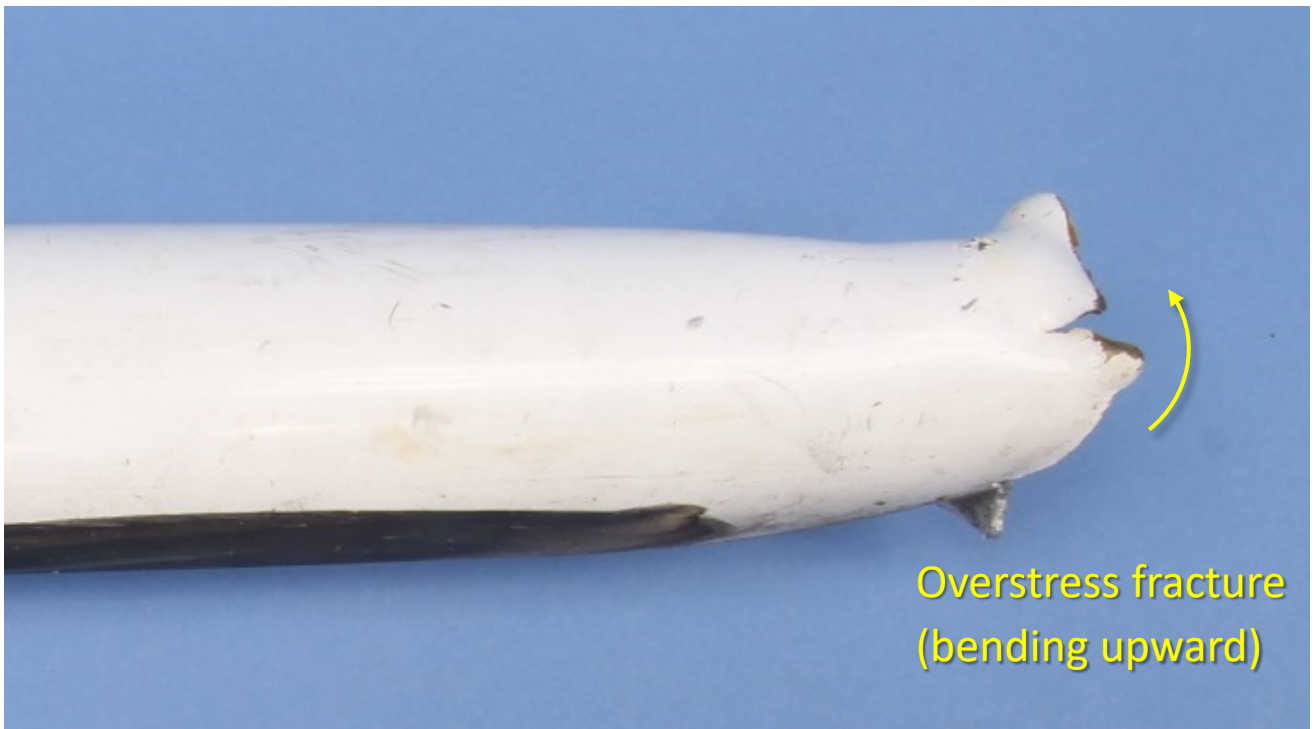
Figure 4 – View of the side of the leg remnant tube fracture surface, showing buckling on the upper side and tension features on the bottom side, consistent with upward bending in the figure.
