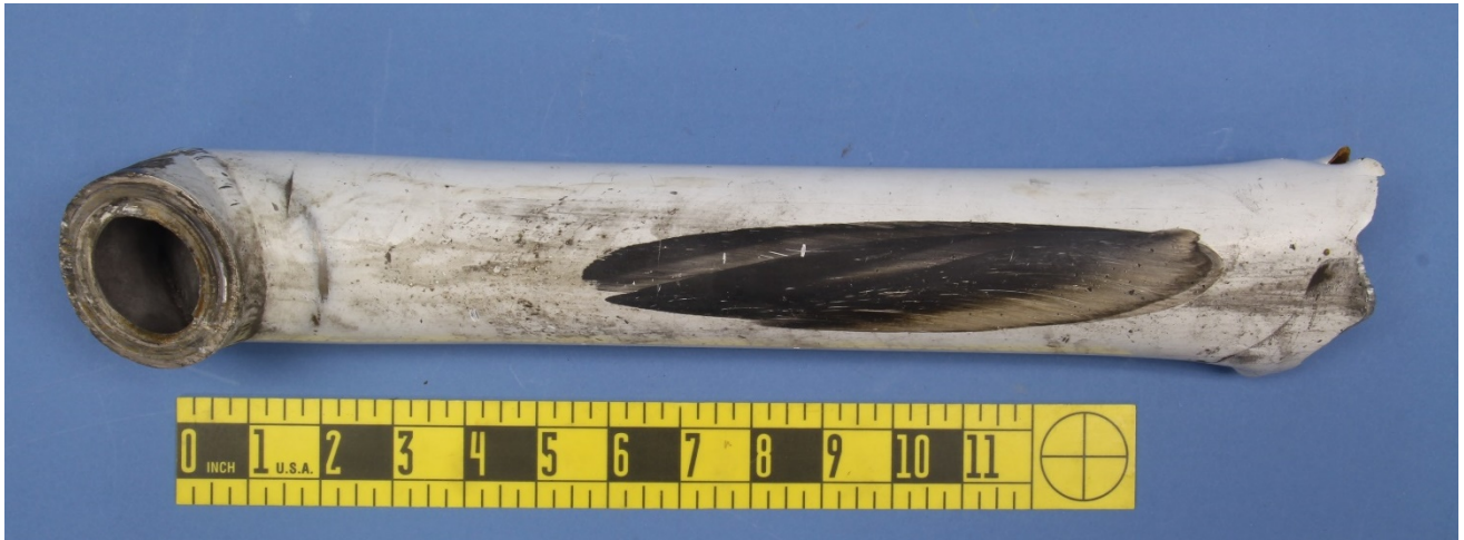
Figure 3 – View of the leg remnant, showing the collar fracture surface and witness marks on the bottom side.
