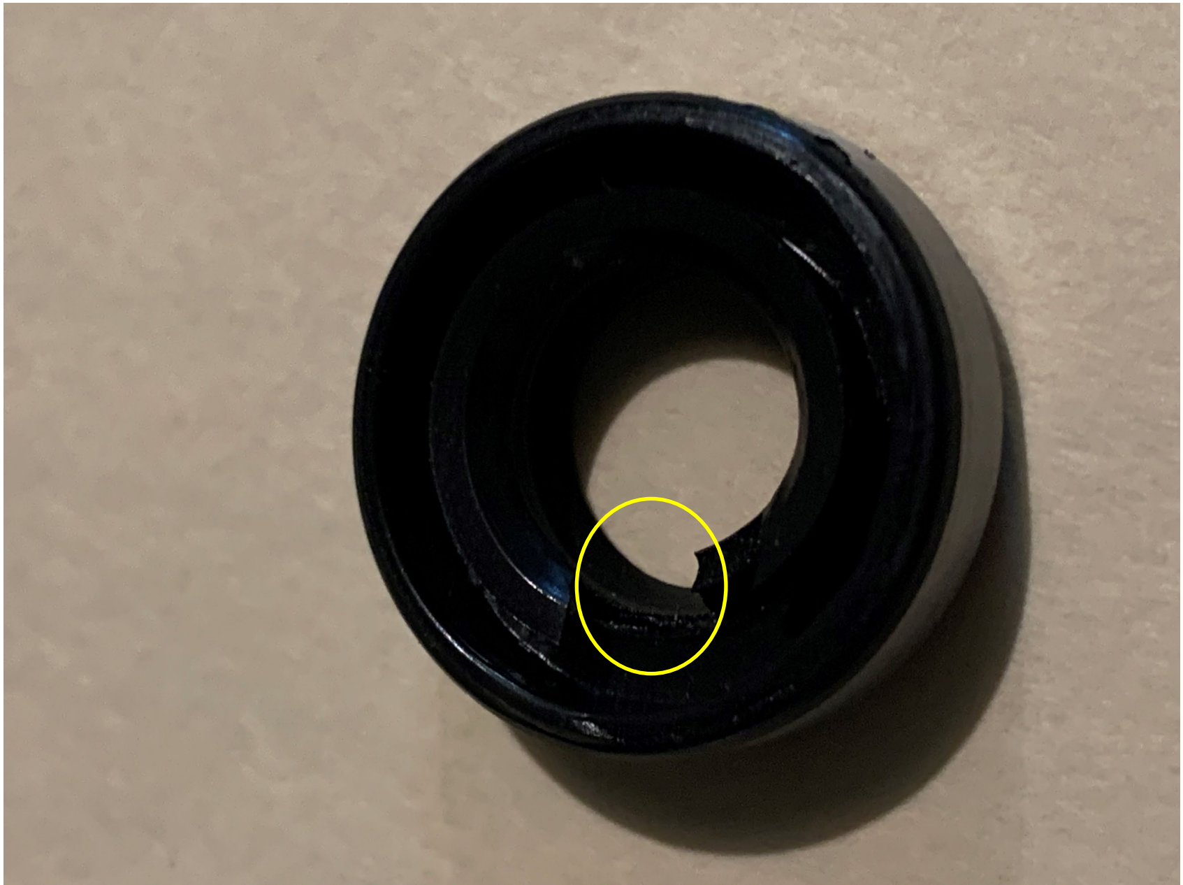
Photo 4 - View of mechanical hydraulic pump seal damage (photo courtesy of the maintenance facility)
