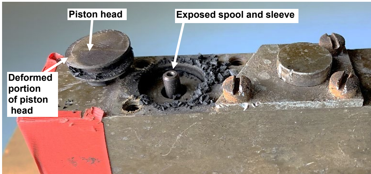
Appendix 2F. Piston head that was extracted from the sequence valve port and exposed top portion of the spool and sleeve.
