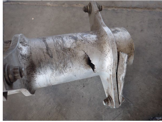
Photo 18. Main drive shaft with puncture indentation.
