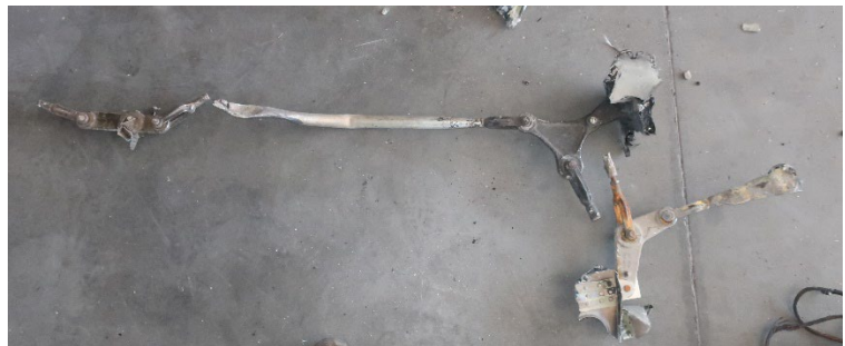
Photo 11 .Elevator control linkages.
