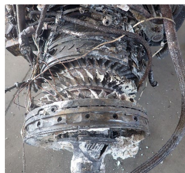
Photo 16. Engine compressor case was consumed by the post-crash fire, revealing the compressor rotor and stator rings.
