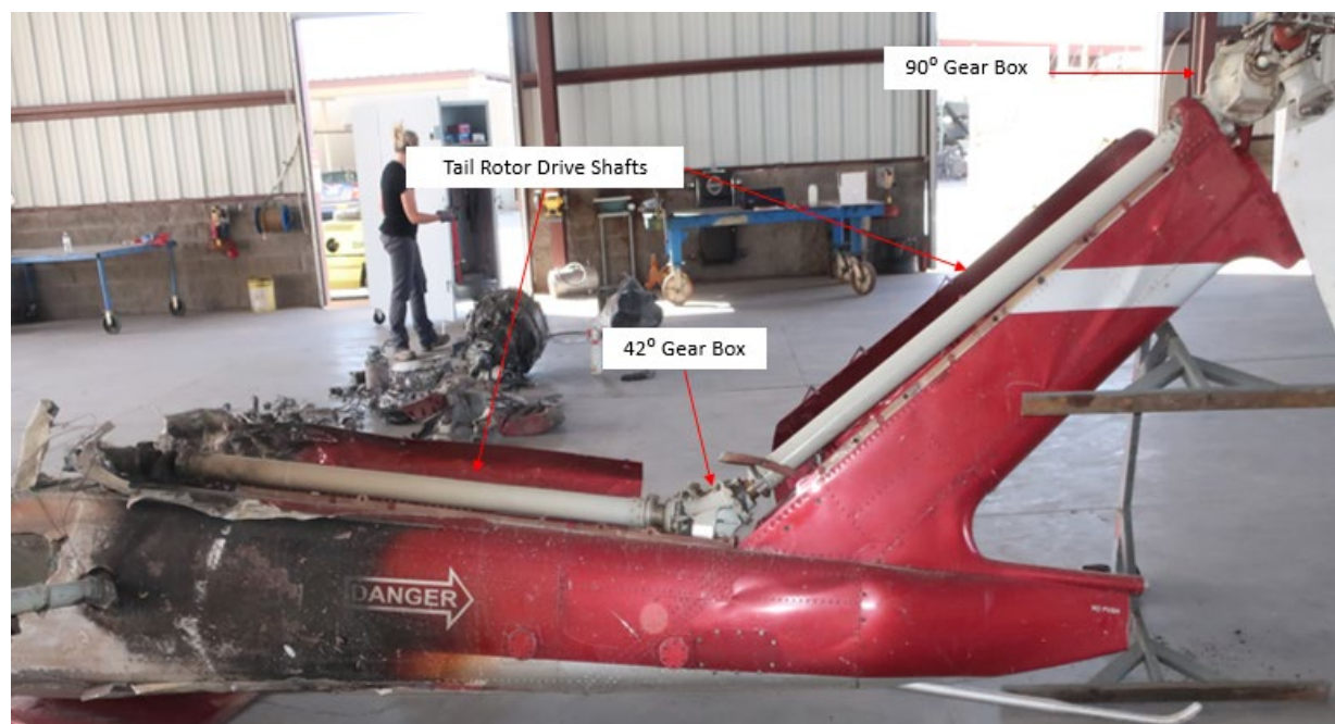
Photo 12. Remnants of the tail boom, vertical fin, tail rotor drives shafts, and tail rotor.
