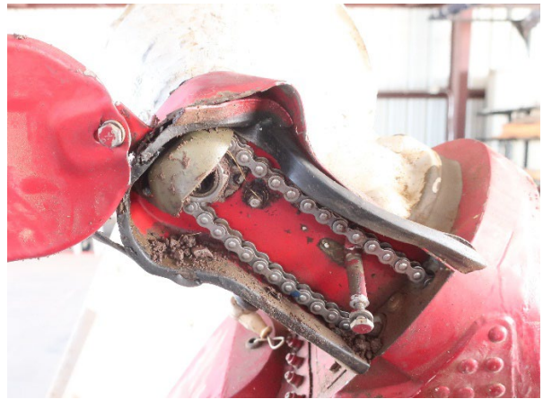
Photo 9 .Tail rotor pitch change control chain & sprocket.
