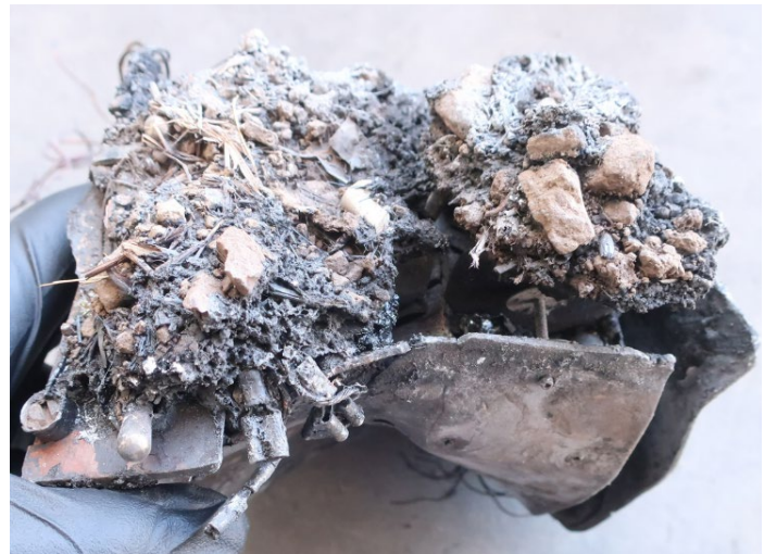
Photo 4. Caution panel as found in the wreckage.
