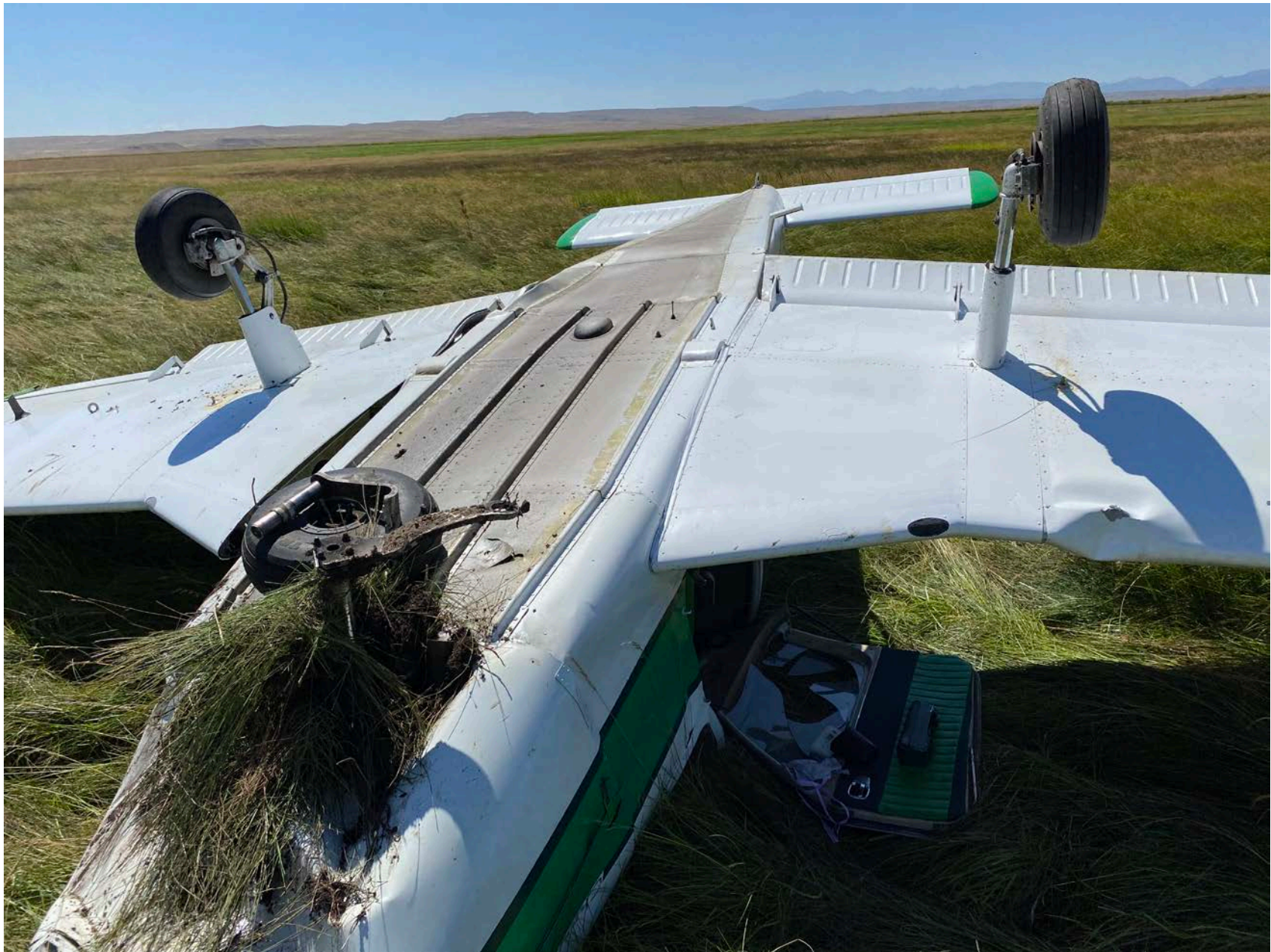
Photo 1 – View of damage to the left wing root and lower fuselage (Courtesy of FAA)
