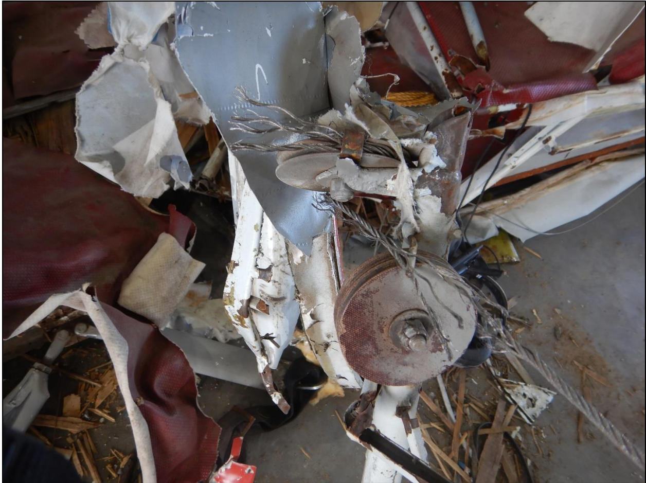
Figure 4-Left aileron cable and pulley assembly.
