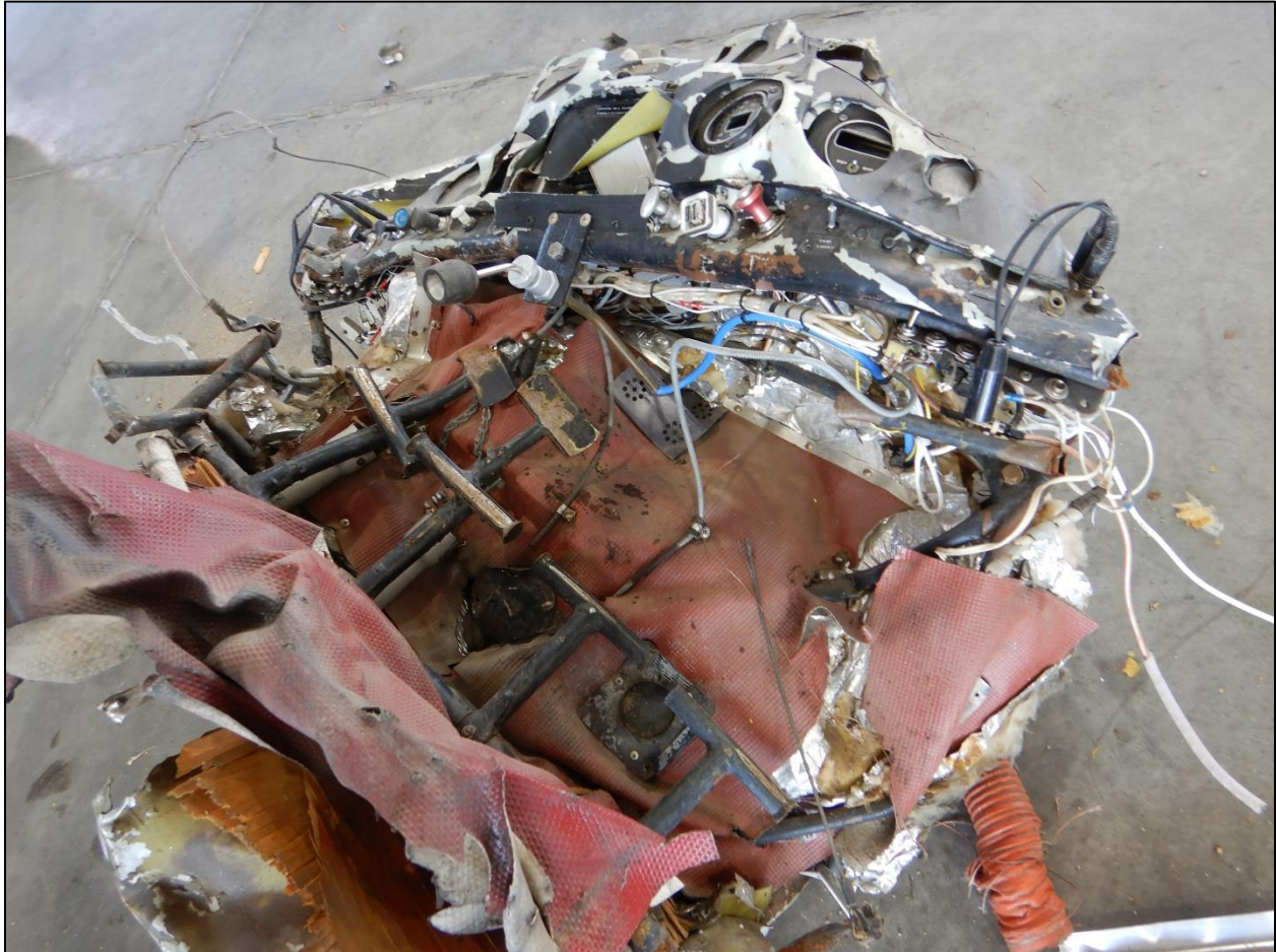
Figure 8-Firewall and the forward fuselage section.
