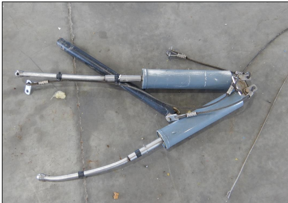
Figure 11-Main landing gear shocks.
