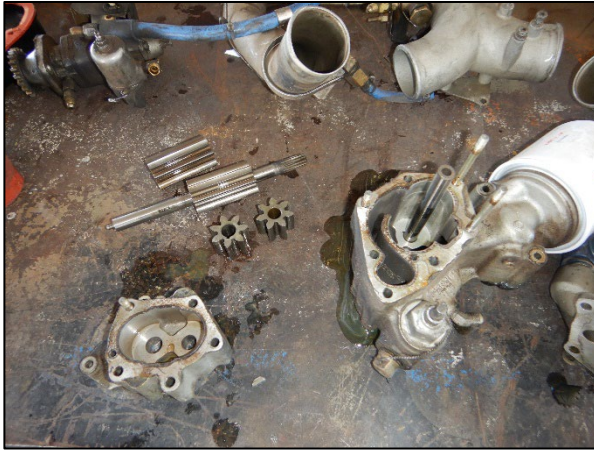
Figure 10-Oil pump and scavenge pump disassembled.
