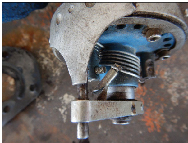
Figure 17-Propeller governor linkage damage.
