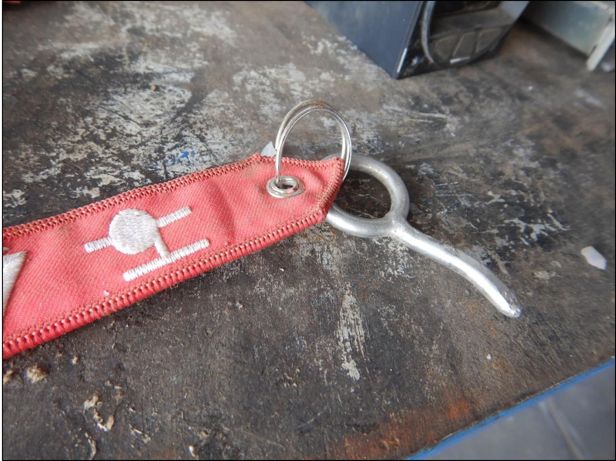
Figure 4-Locking pin and remove before flight tag.
