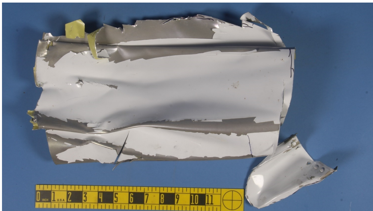
Figure 1 – Sections of the dented wing skin assembly, viewed from the exterior side, as received.
