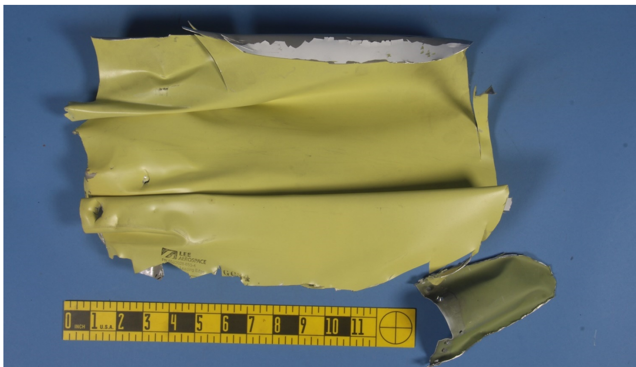
Figure 2 – Sections of the dented wing skin assembly, viewed from the interior side, as received.
