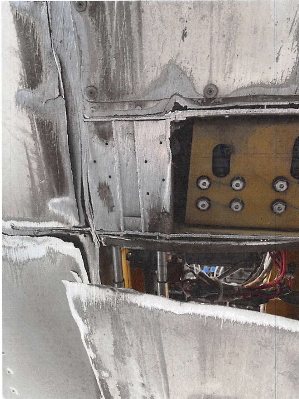
Photo 1 - Structural damage to the undercarriage keel beam
