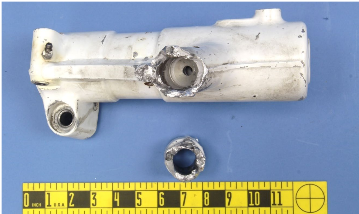
Figure 4 – View of the two fracture surface of the fractured trunnion boss, after removal of tape and separation.
