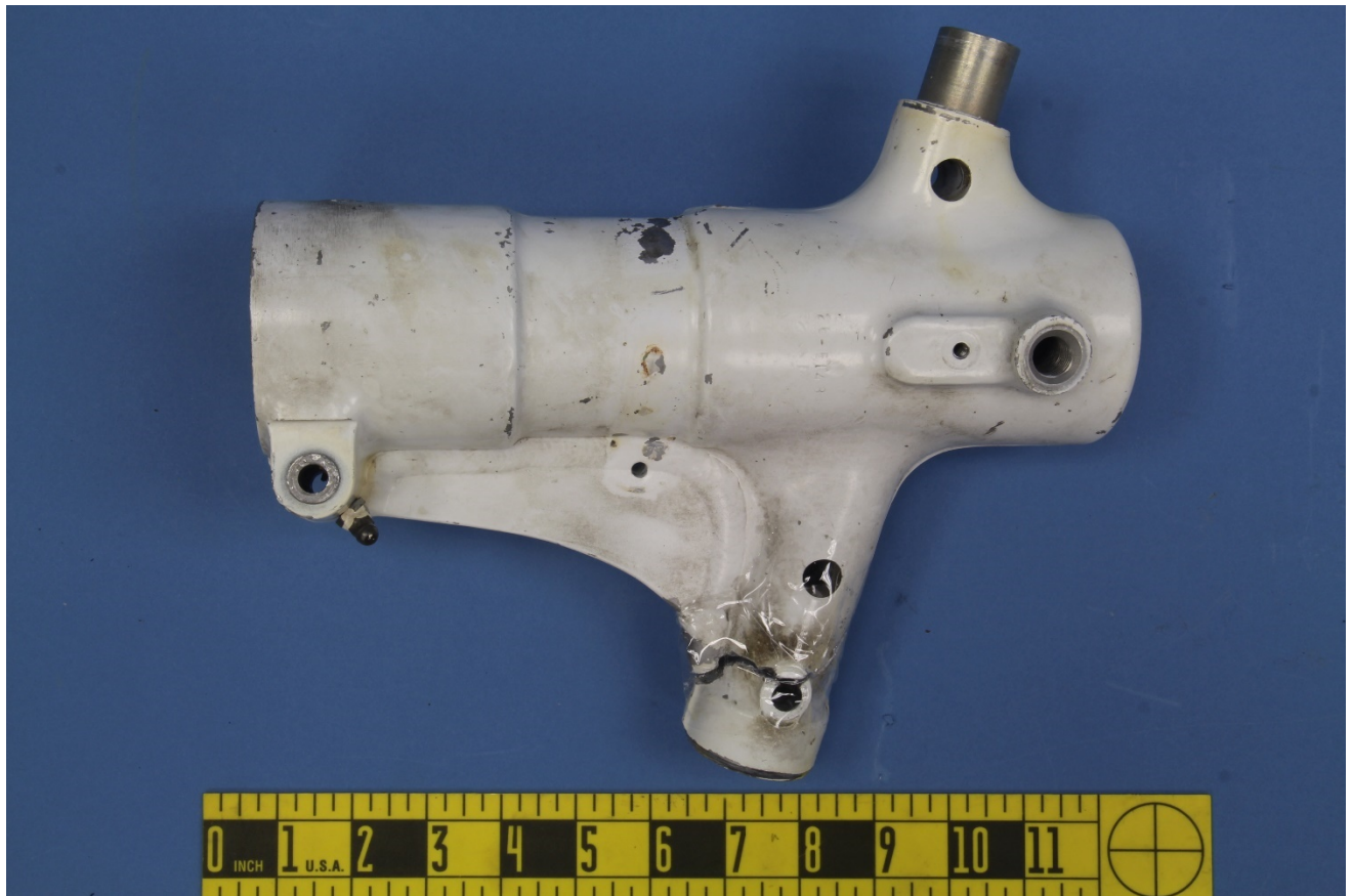
Figure 2 – View of the trunnion from the reverse side of Figure 1, as received.
