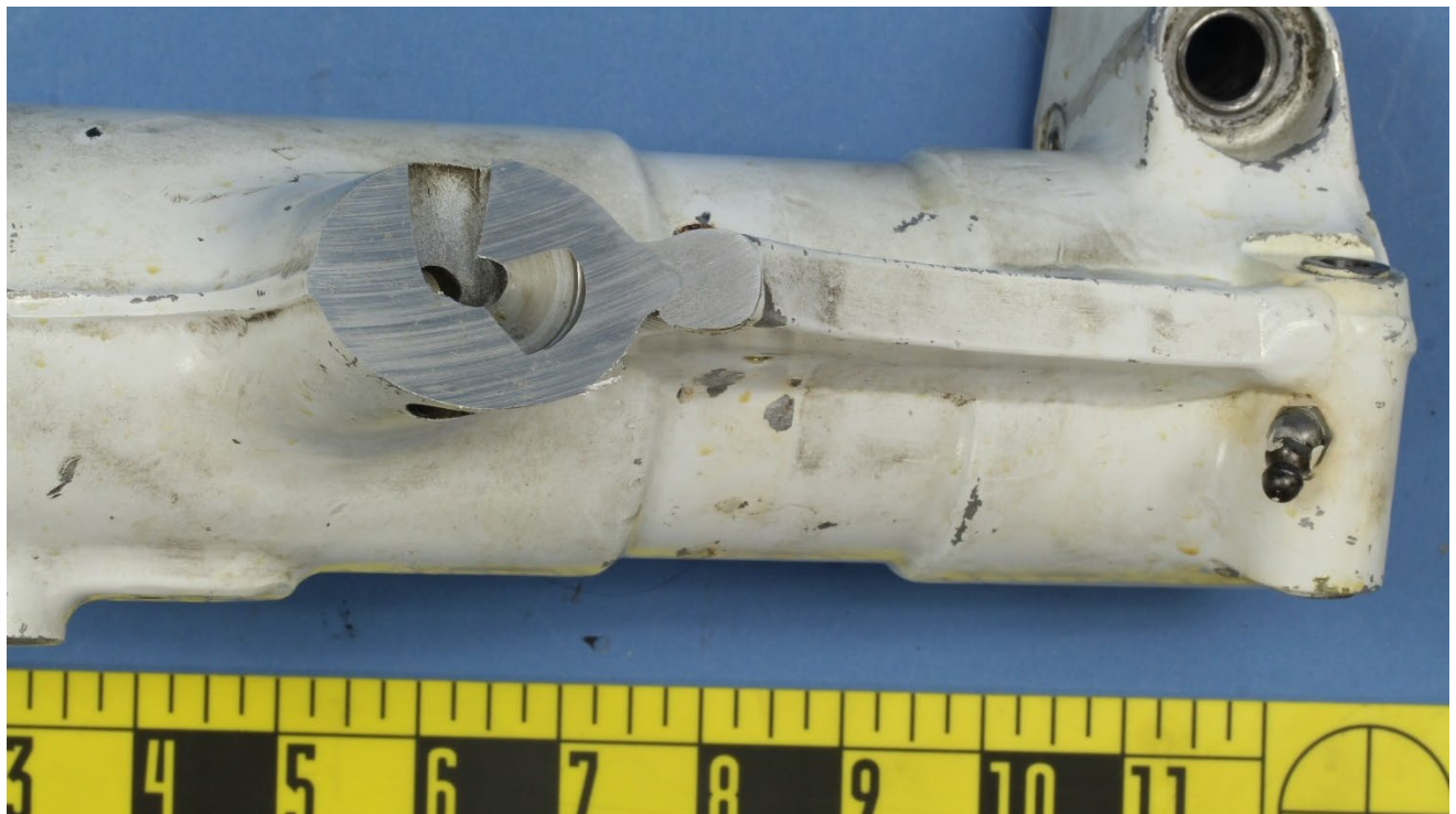
Figure 12 – View of the trunnion after sectioning of the inner fracture surface of the boss, showing the general cross-section dimensions of the joint.
