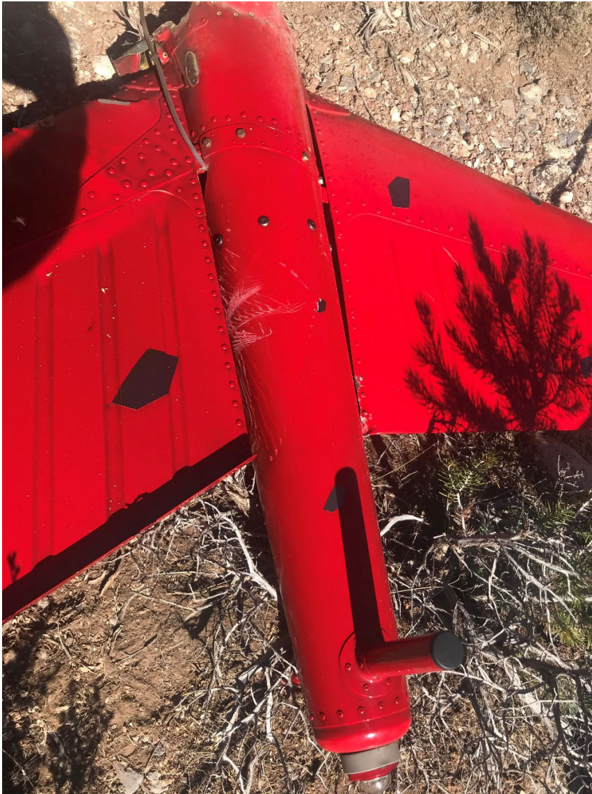
Photo 5 Vertical Fin Note cable braiding signatures on the left side
