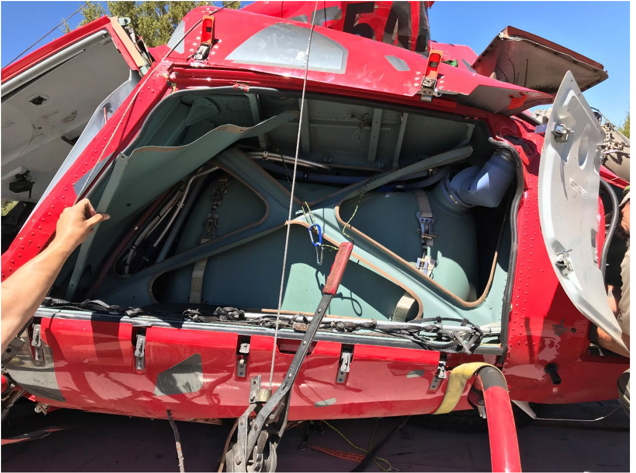
Photo 7 View of Fuel Tank
