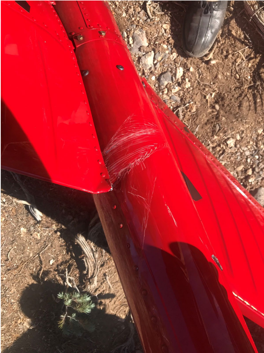
Photo 6 Close up View of the Cable Braiding Signatures
