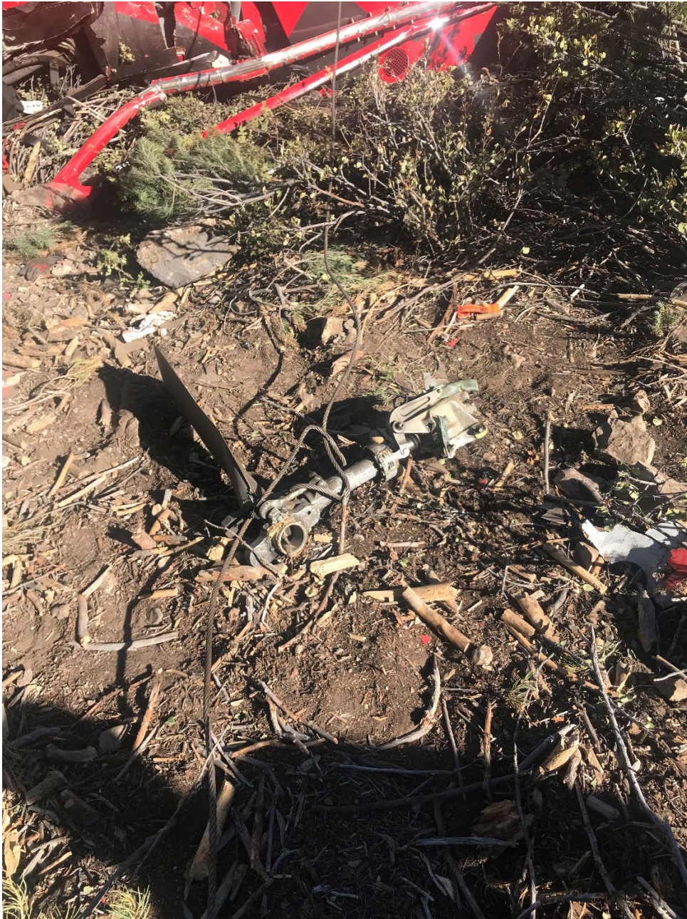
Photo 4 - Long Line wrapped around Tail Rotor
