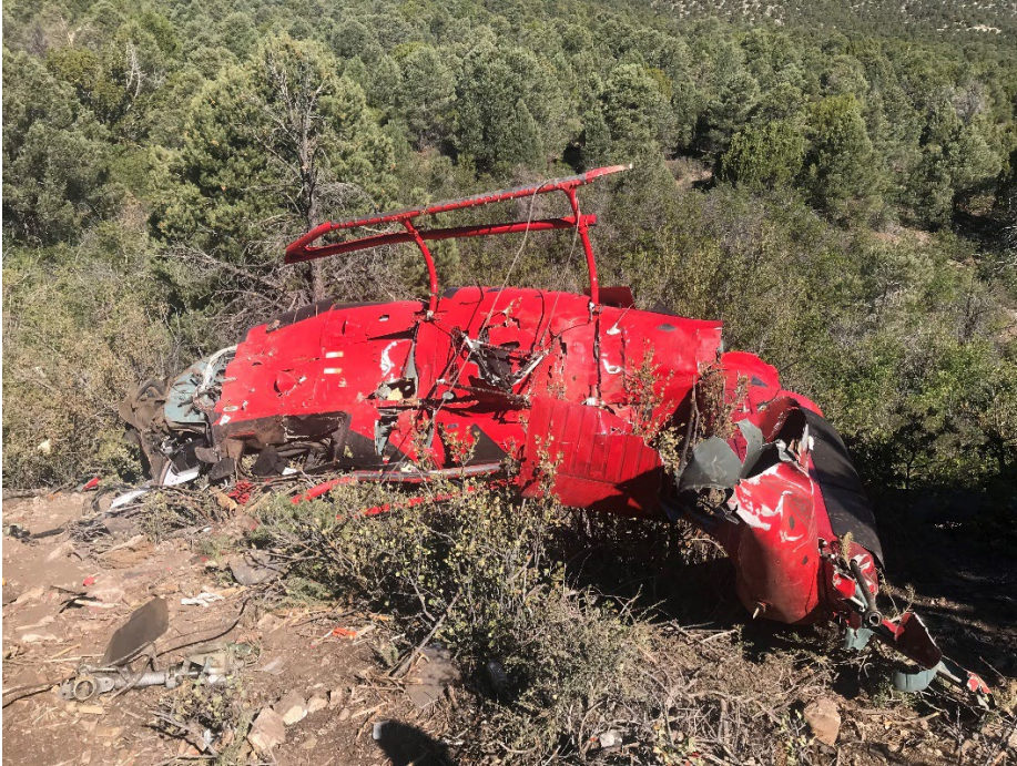
Photo 2 – Close up View of Undercarriage Note Long Line Cable wrapped around the upper skid
