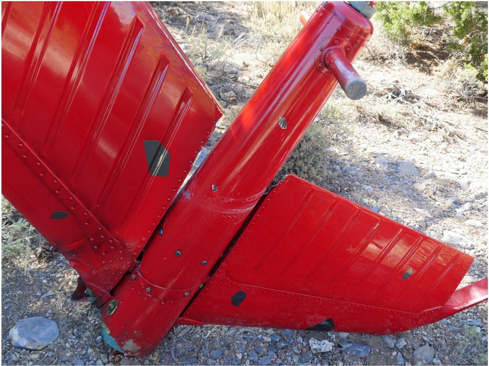
Photo 5 – Cable Braiding Signatures on Vertical Fin (Photo Courtesy of FAA)
