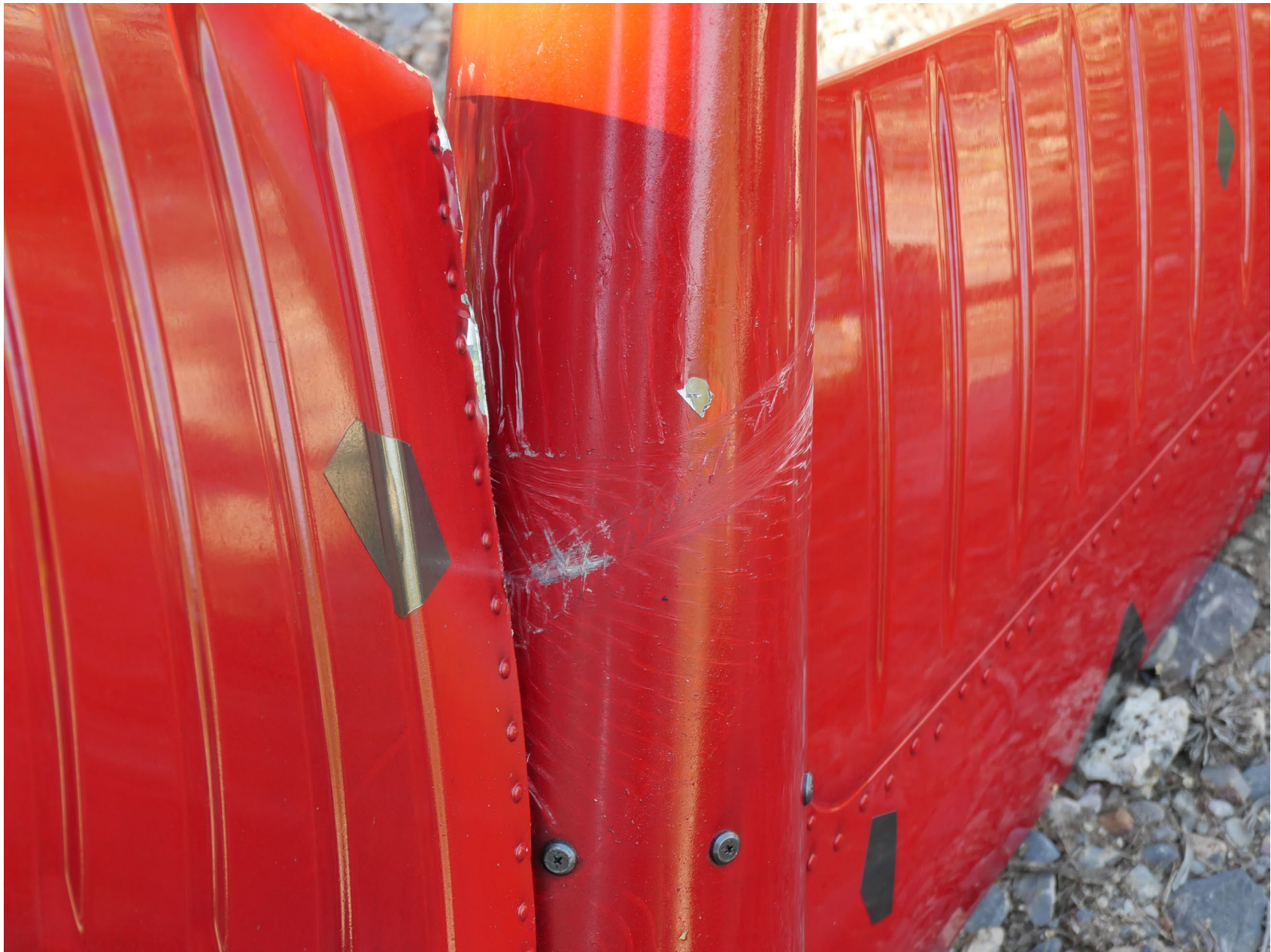
Photo 6 – Close up View of Cable Braiding Signatures (Photo Courtesy of FAA)
