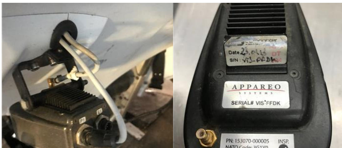
Figure 4. The accident unit, as noted in the wreckage, post-accident.
