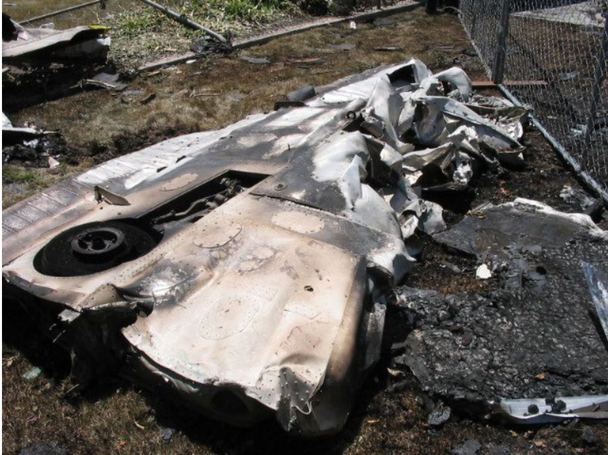
Figure 7. Underside of the right wing, showing leading edge, landing gear, and flap. Photo courtesy of Piper Aircraft.
