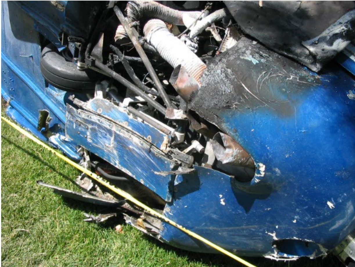
Figure 15. Underside view, showing the retracted nose landing gear. Photo courtesy of Piper Aircraft.
