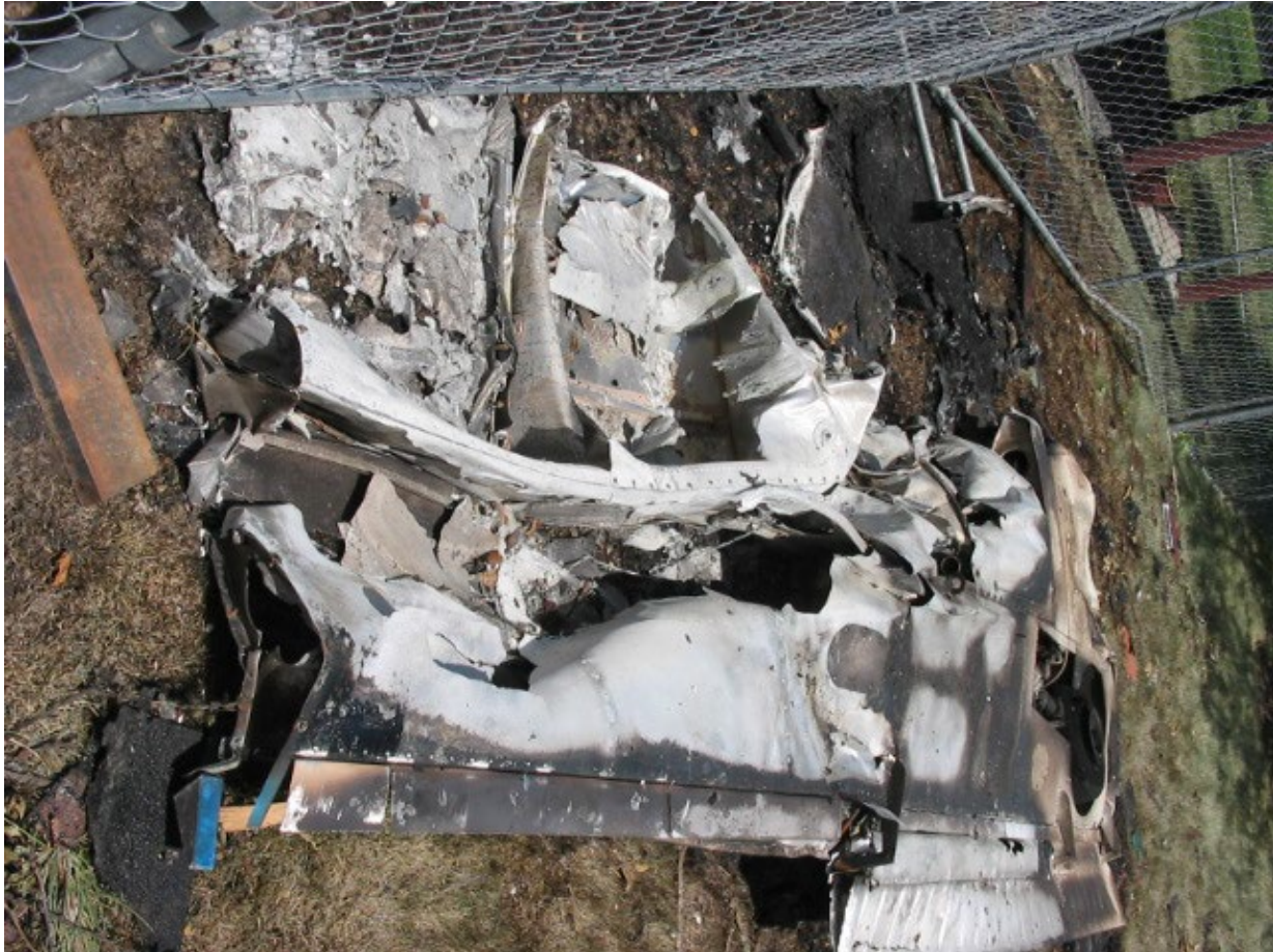
Figure 8. Under side of the right wing, showing the flap. Photo courtesy of Piper Aircraft.
