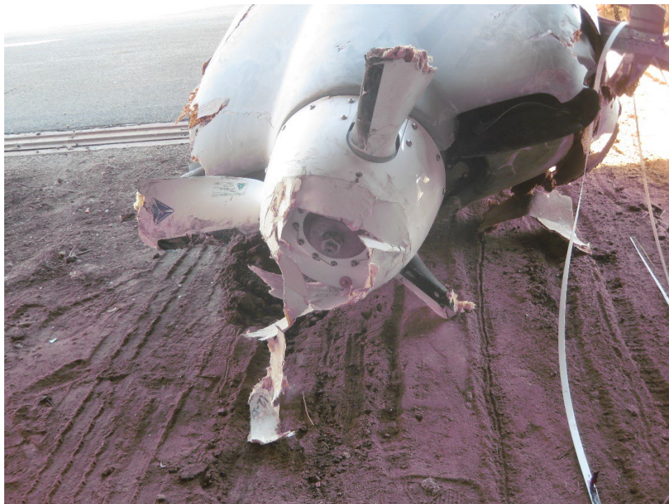
Figure 4: Damage to the Spinner and Propeller Blades
