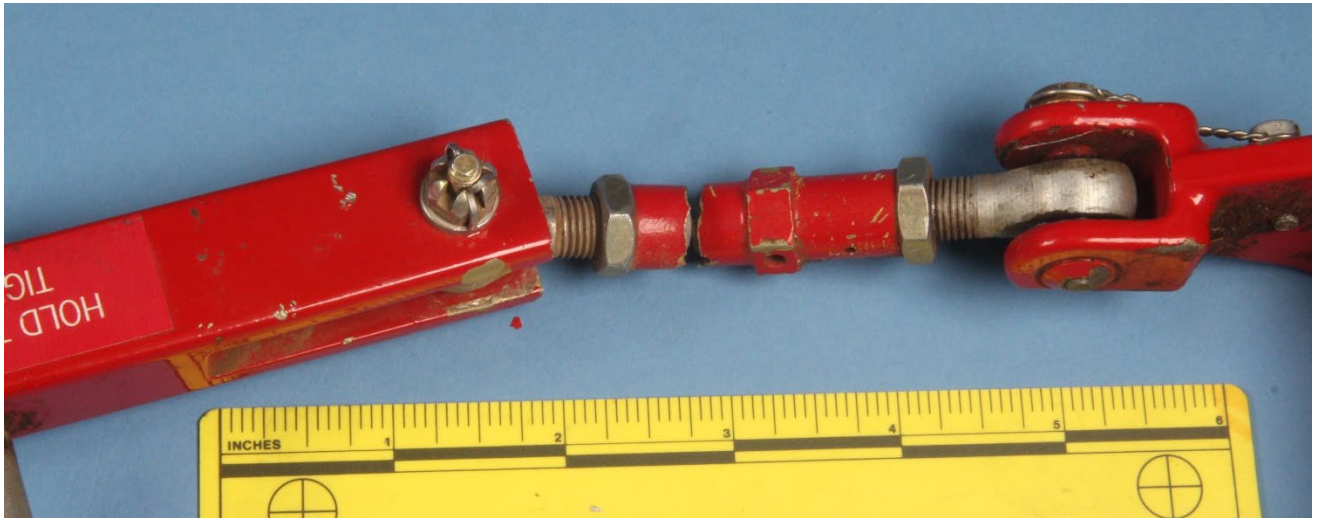
Figure 6 – Views of the fractured remnants of a pitch change link, as received.
