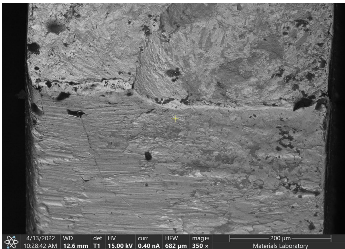
Figure 26 – BE micrograph of an angled view of the crack initiation sites.
