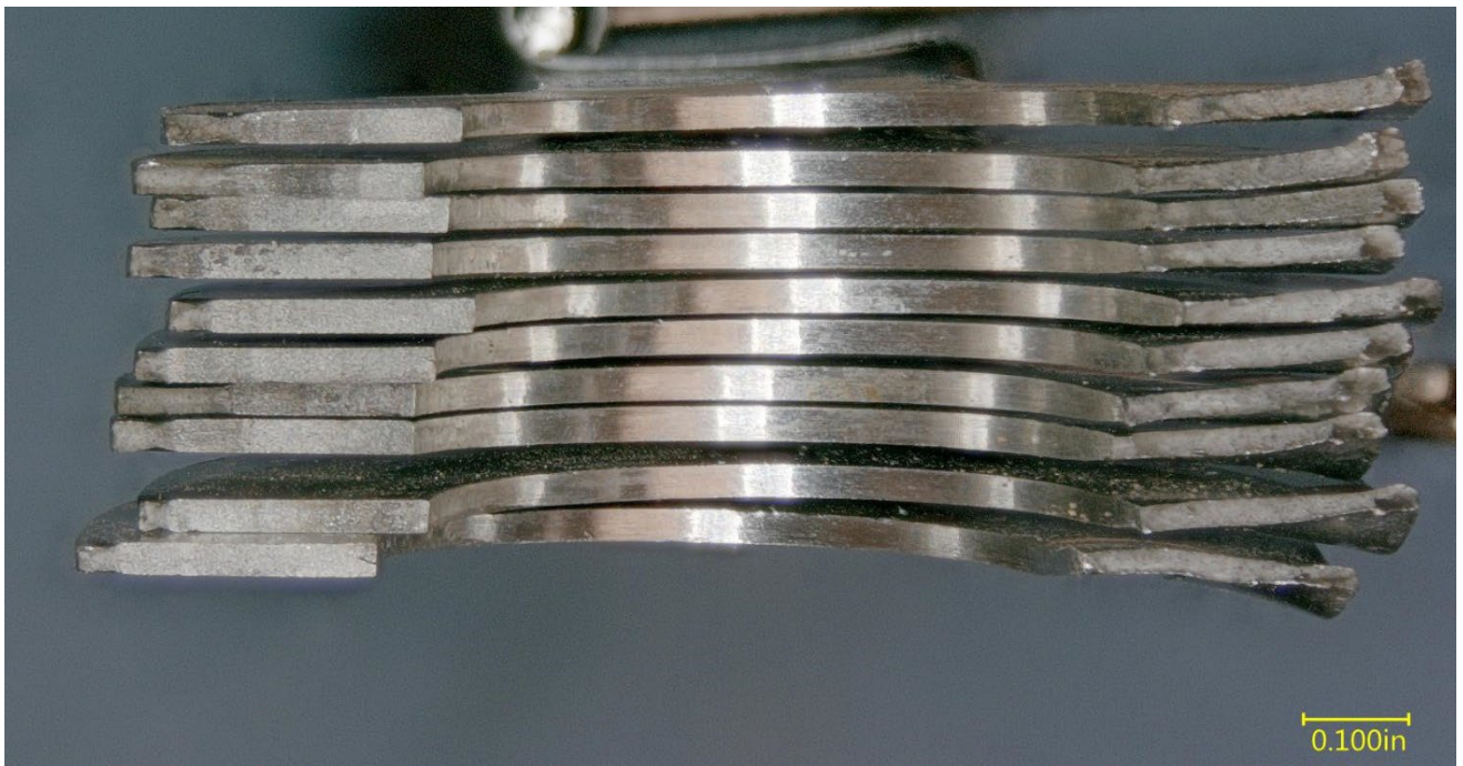
Figure 16 – View of the fracture surfaces of the bundle of TT straps in Figure 12.
