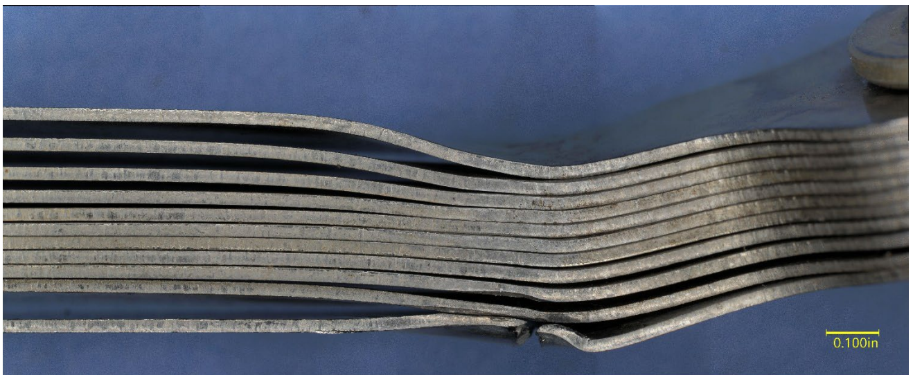
Figure 12 – Side view of the TT strap bundle in Figure 11, showing the fractured strap facing downward at the bend in the set.
