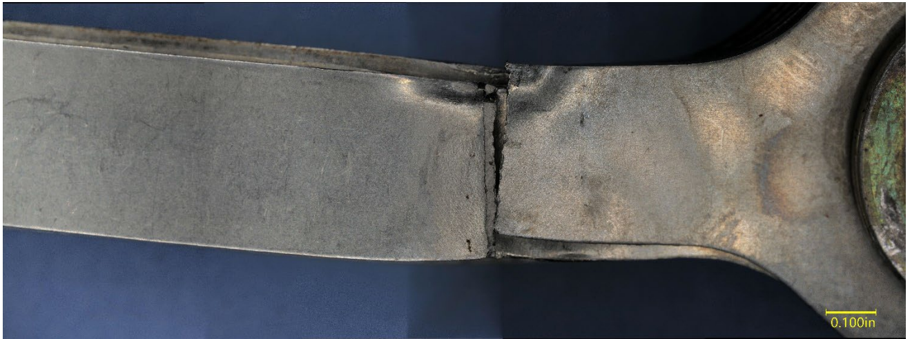
Figure 11 – View of the deformed and fractured TT strap bundle from the second blade assembly, showing necking and buckling near the fracture of the outer strap.
