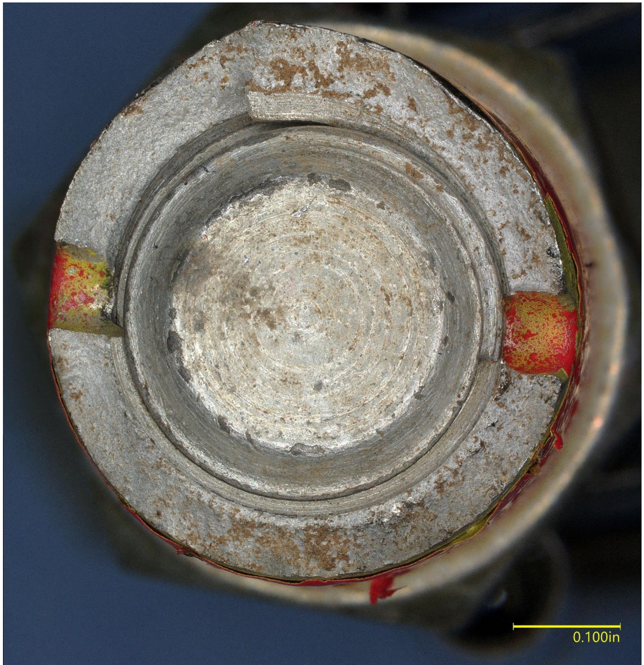
Figure 8 – View of the rod end fracture surface.
