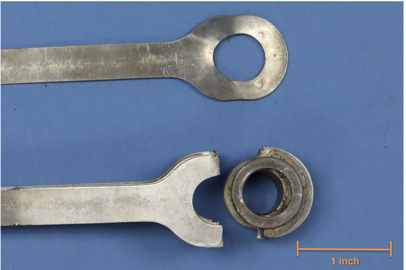
Figure 14 – The fractured ends of 10 of the 11 TT straps in the bundle, along with the one intact strap, exhibiting elongation.
