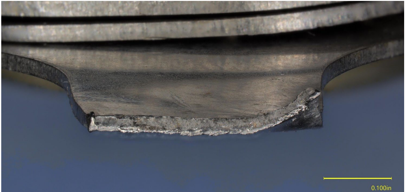
Figure 13 – View of the fracture surface of the fractured strap in Figure 11, showing a slanted orientation.
