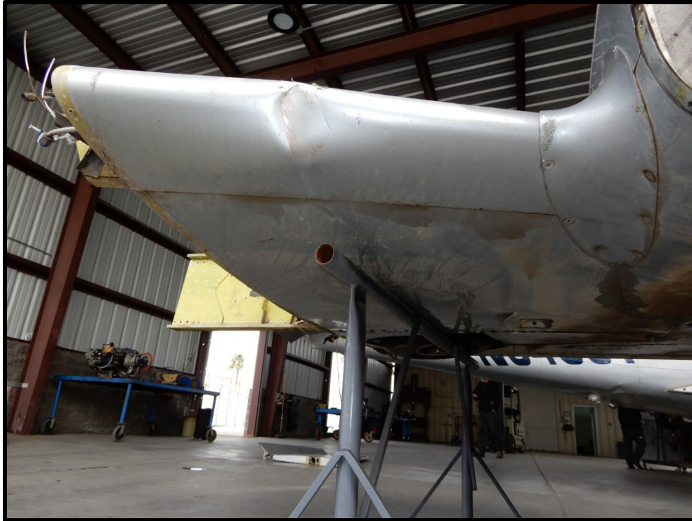
Photo 9. Left wing with damage to the leading edge.
