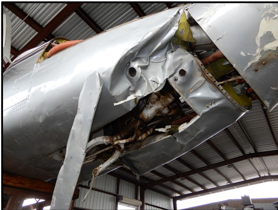
Photo 16. Right side of fuselage, showing damage to the nose cone and nose gear bay.
