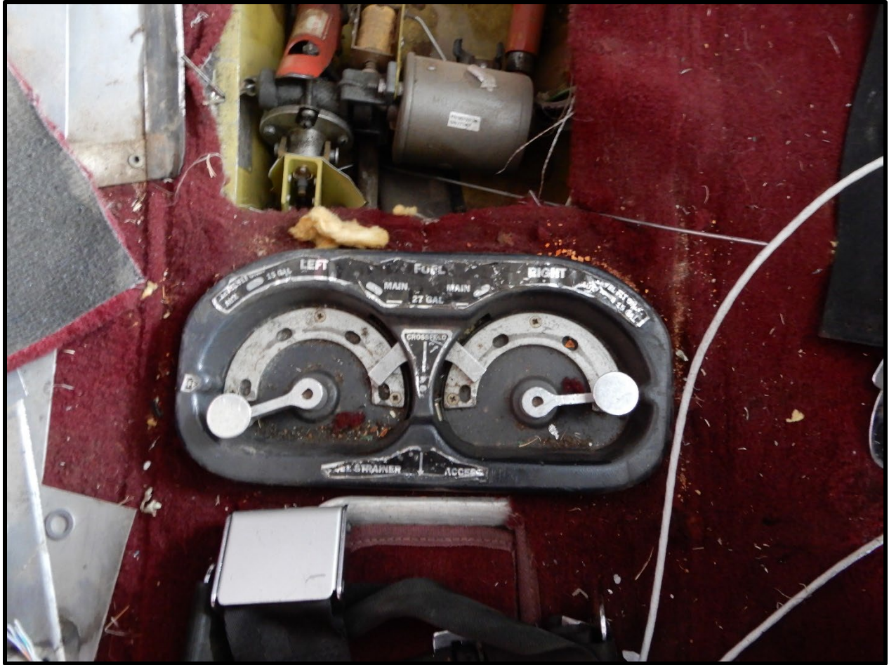
Photo 19. Fuel selector switches.
