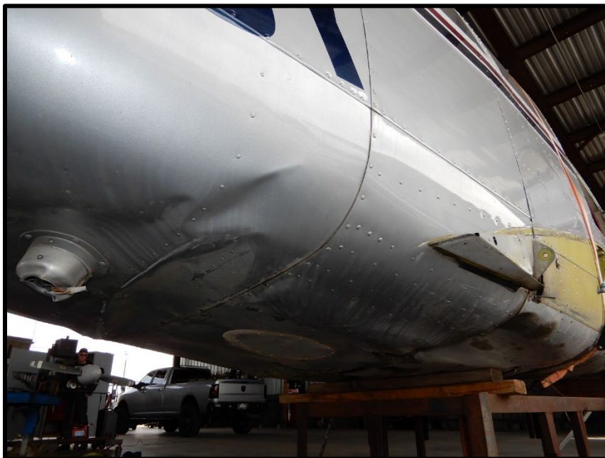
Photo 14. Right side of fuselage, showing damage to underside.
