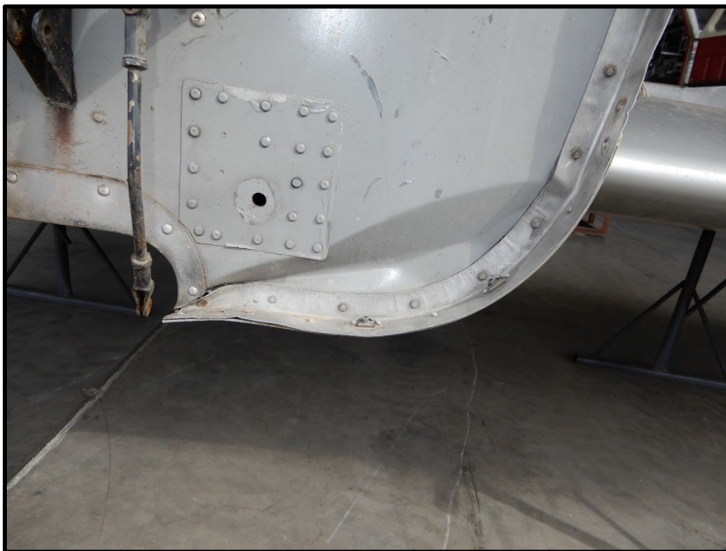
Photo 8. Left wing engine firewall.
