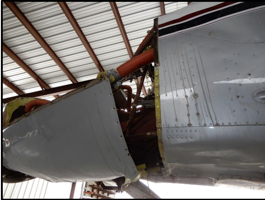
Photo 17. Left side, showing damage to the nose gear bay area.
