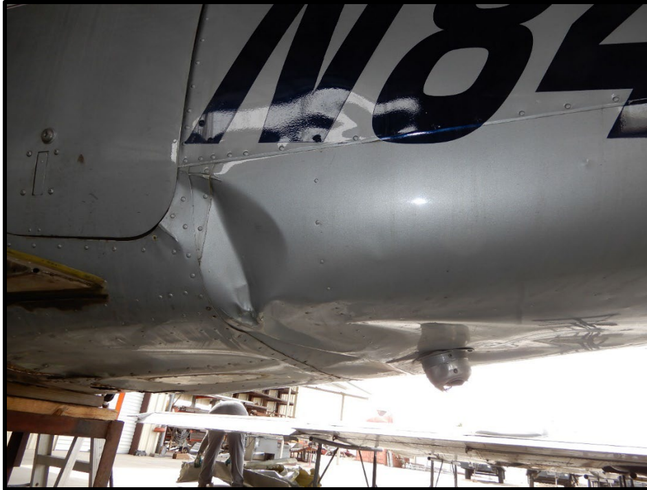
Photo 15. Left side of fuselage, showing damage to underside.
