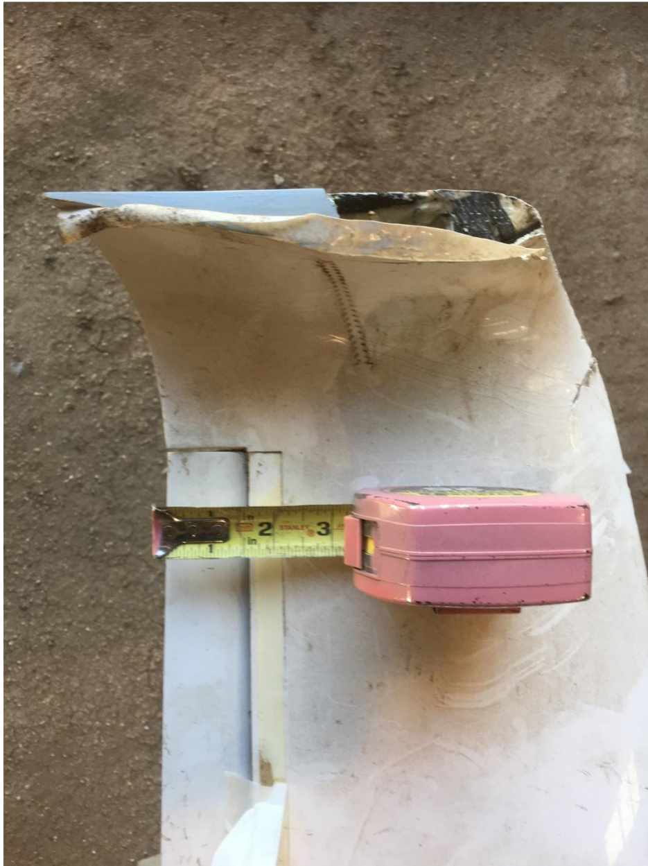
IMG_1988: Width of aileron on 15m wing tip extension ("mini-aileron")
