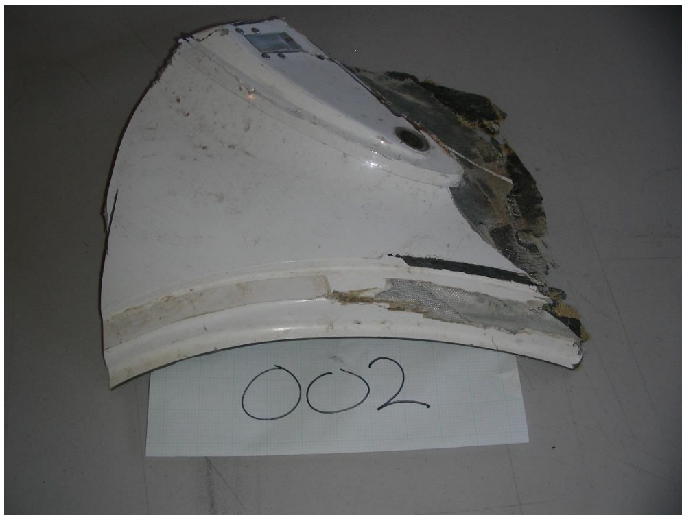
002: Left Wing Rocker and Housing Assembly (outside view)
