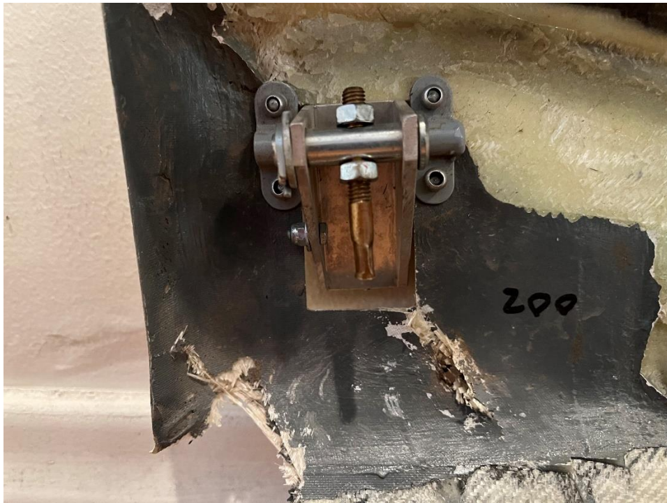
Image_2833: L/H rocker close-up view showing side profile of crimp on brass tube.
