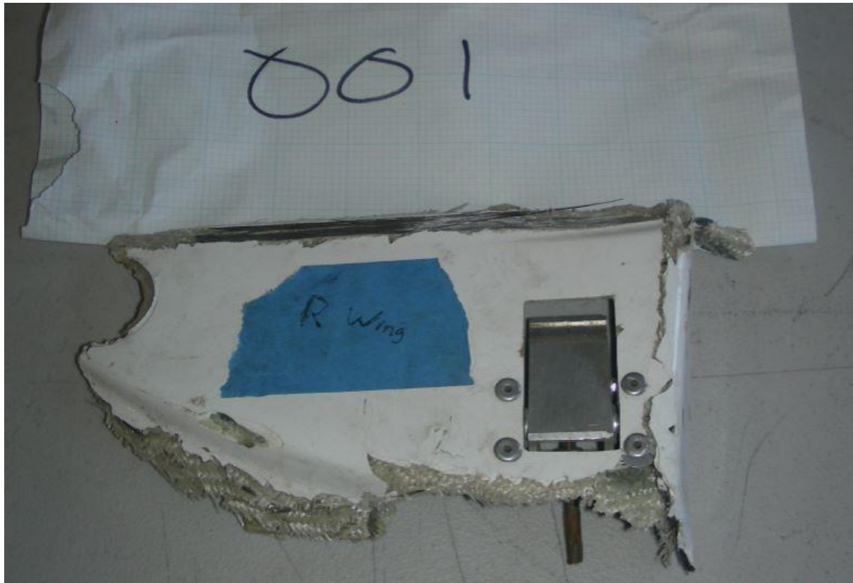
001: Right Rocker and Housing Assembly (outside view)
