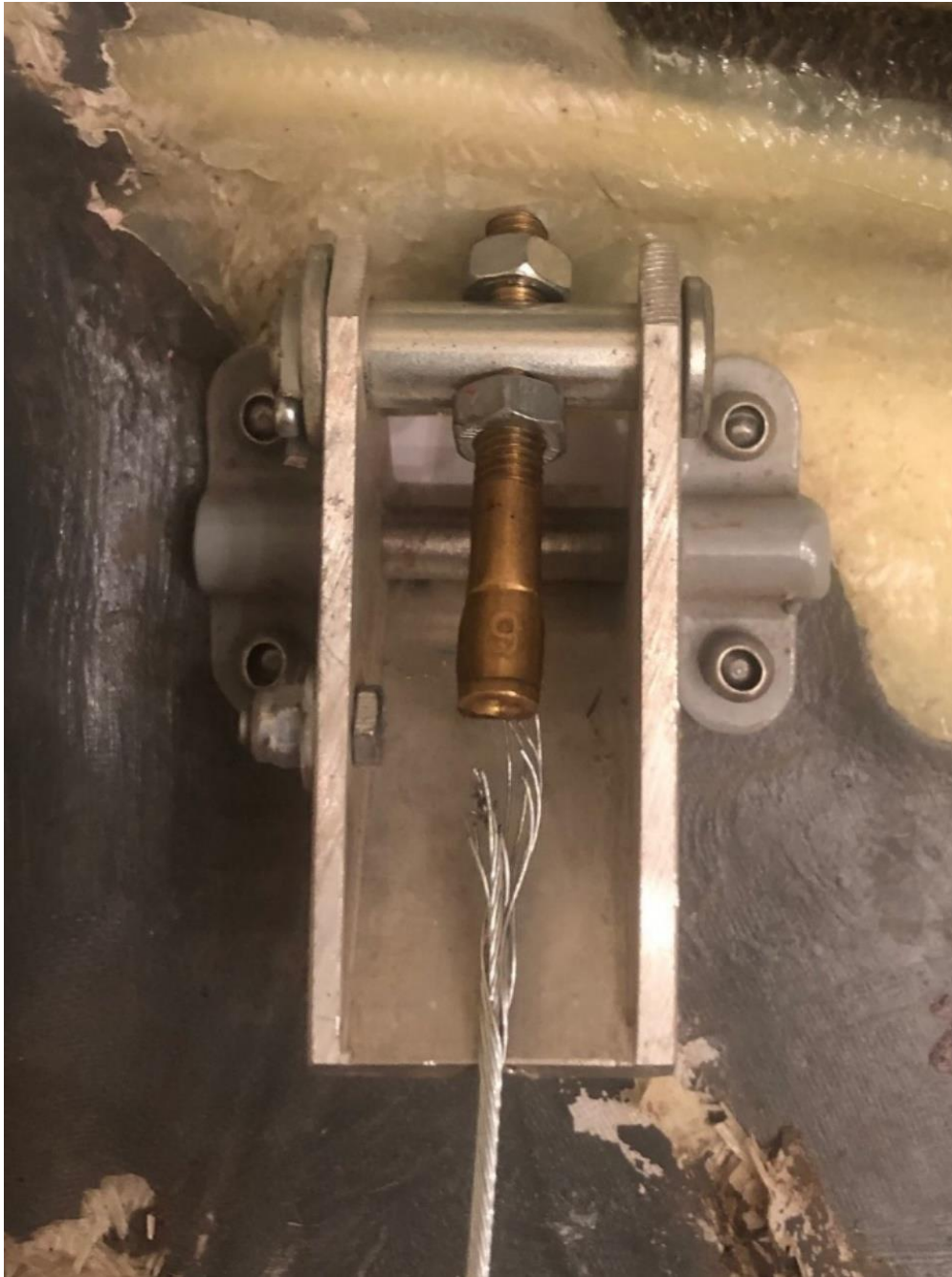
Image_6094: L/H Bowden cable pulled out from the brass tube.
