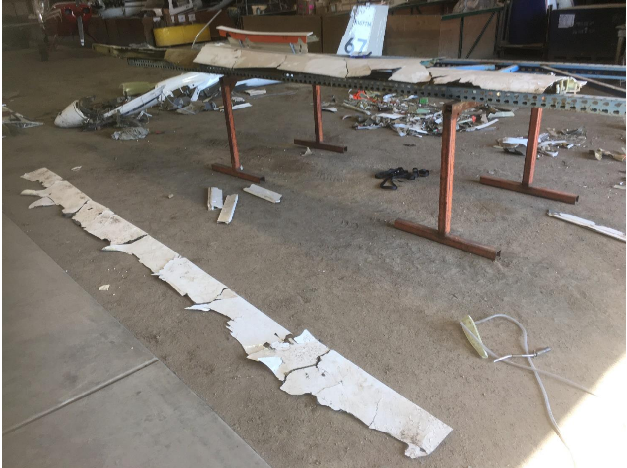
Image_1985: Reconstructed fragments of lower and upper parts of left inner wing.
