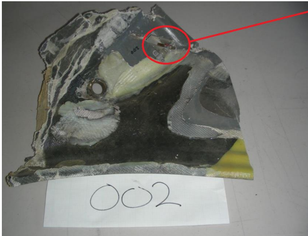
002: Left Wing Rocker and Housing Assembly (inside view)
