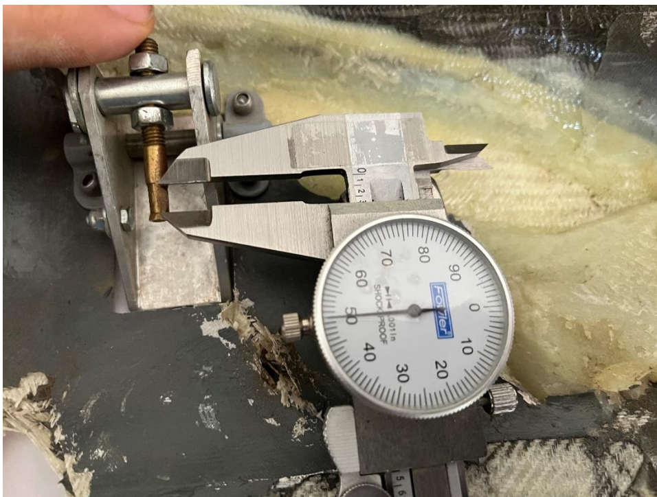
Image_2836: Crimp on brass tube measures 0.25 inches (6mm) in size.
