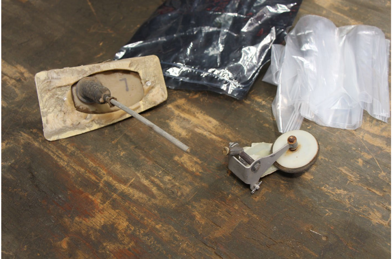
Photograph 7: Left wing water ballast valve
