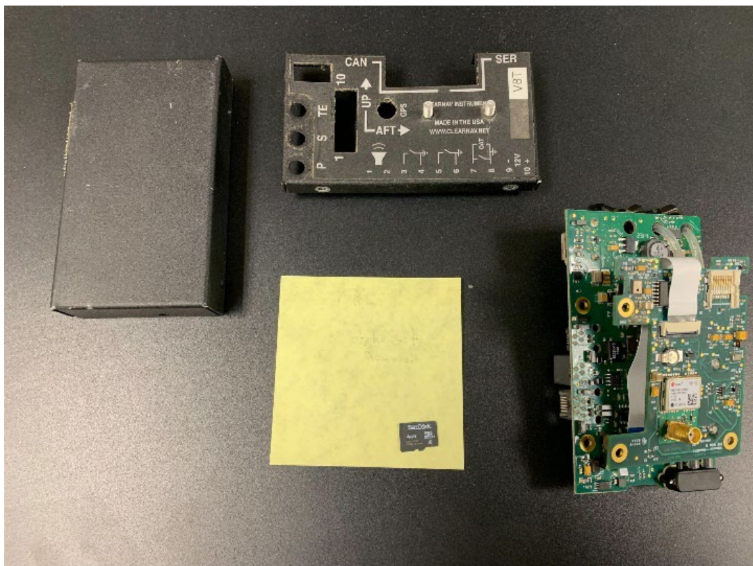
Figure 2. Disassembled air data computer, Micro SD card
