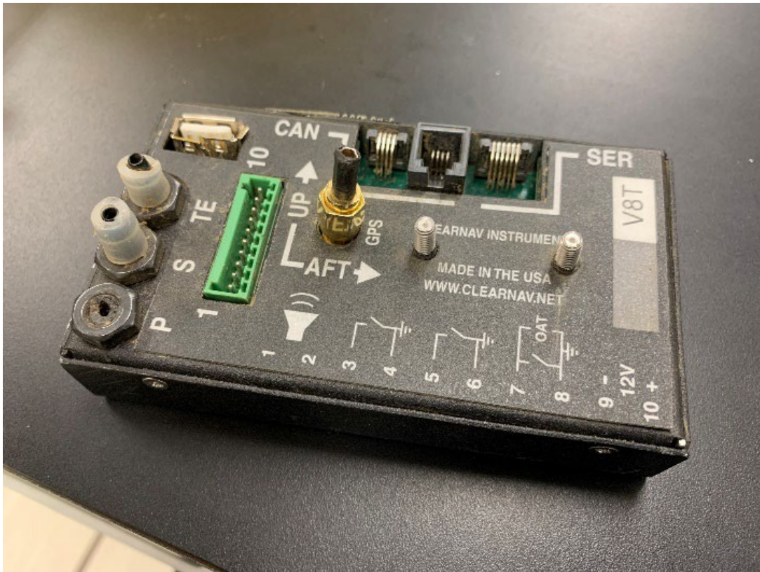
Figure 1. Damaged exterior of air data computer.
