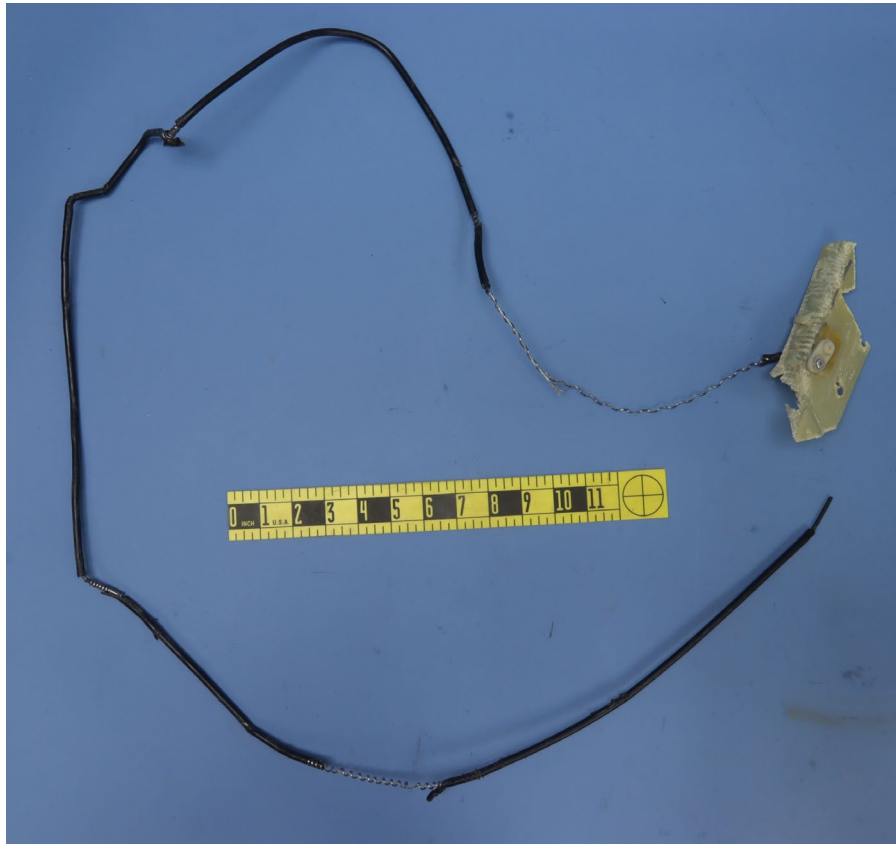
Figure 3: Portion of Bowden cable with sheathing and a fragment of fuselage (as received).
