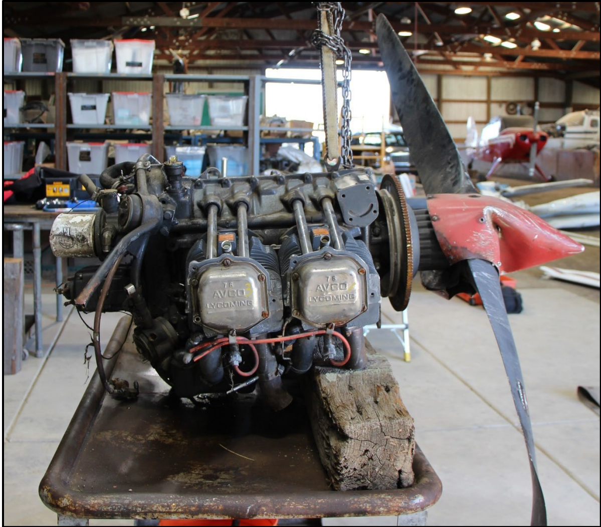
Photograph 3: Engine with Baffling and Exhaust Removed
