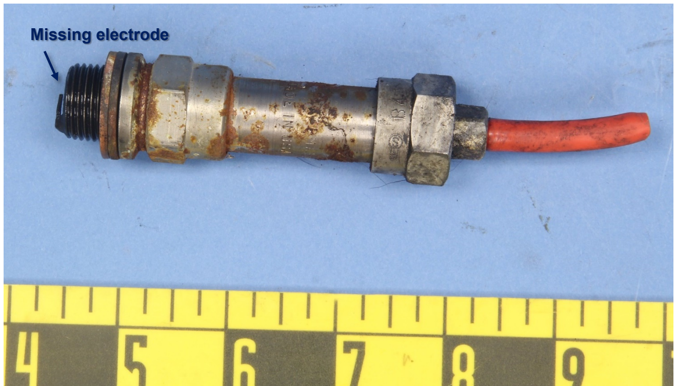
Figure 1 – View of the spark plug and wire remnant, as received.
