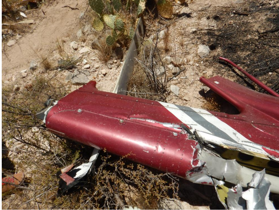
Figure 41. Damage between 45° Gearbox and 90° Gearbox and Damaged Tail Rotor
