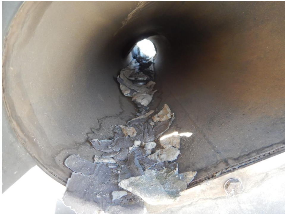
Figure 38. Melted Tail Rotor Drive Shaft
