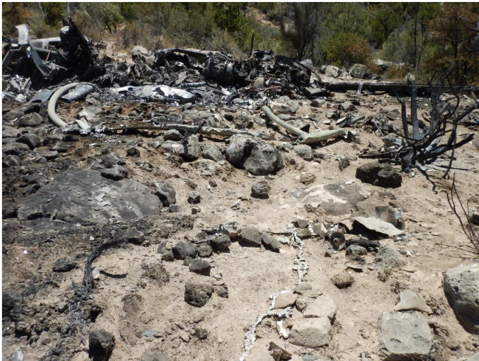
Figure 22. Re-Solidified Melted Metal Running Downhill
