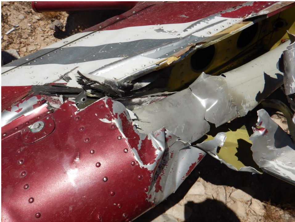
Figure 40. Piece of Tail Rotor Blade Embedded in Vertical Tail
