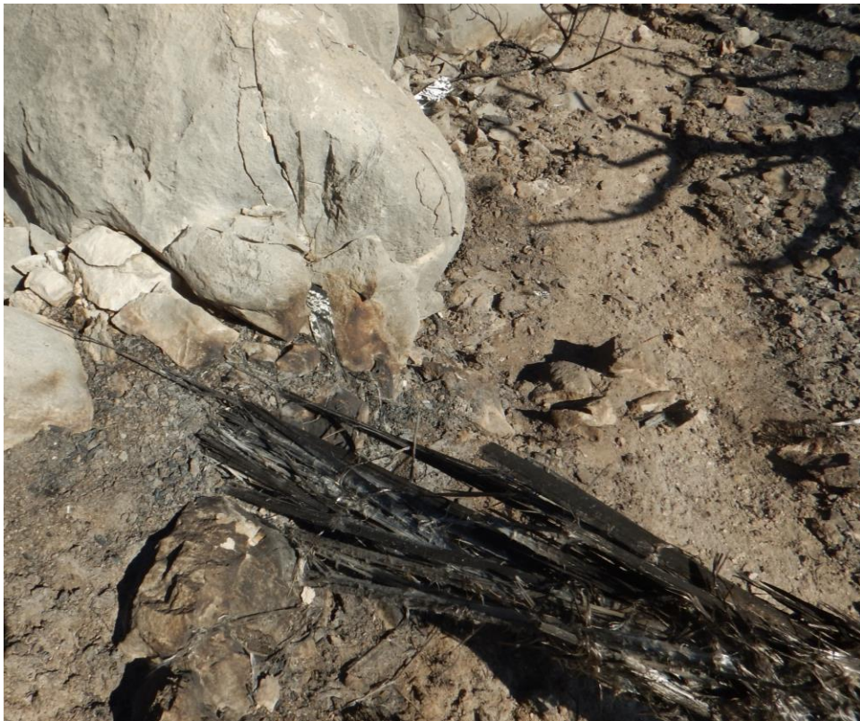
Figure 14. Scarring and Fracturing on Rock by Blade B Tip
