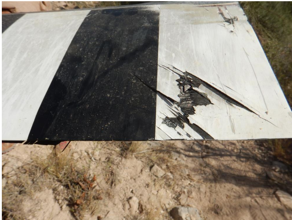
Figure 42. Impact Damage on Intact Tail Rotor Blade Side 1
