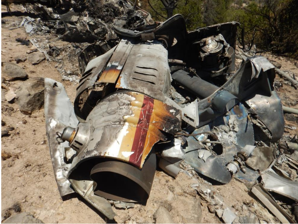
Figure 31. Engine Rolled CCW (Aft Looking Forward) Slightly Uphill
