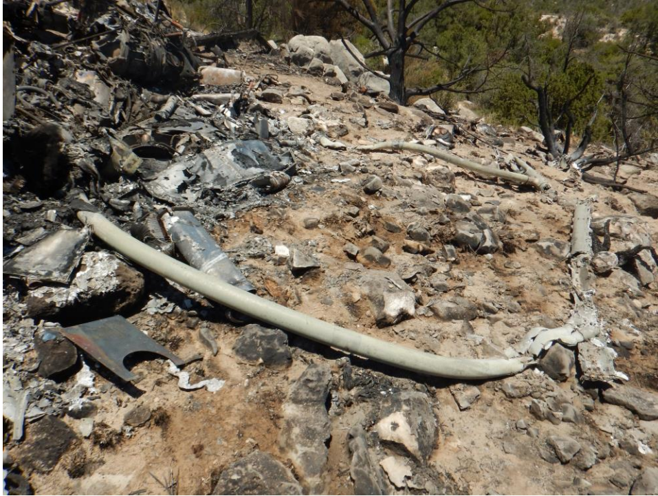
Figure 25. Skids Displaced on Right Side of Helicopter
