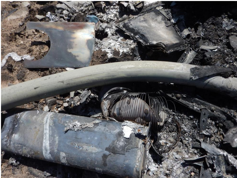
Figure 26. Scrape Marks on Aft Skid Crossmember
