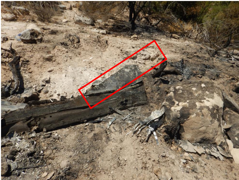
Figure 6. Ground Scar Near Tip of Main Rotor Blade A
