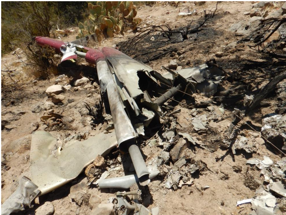
Figure 36. Tail Section Separation
