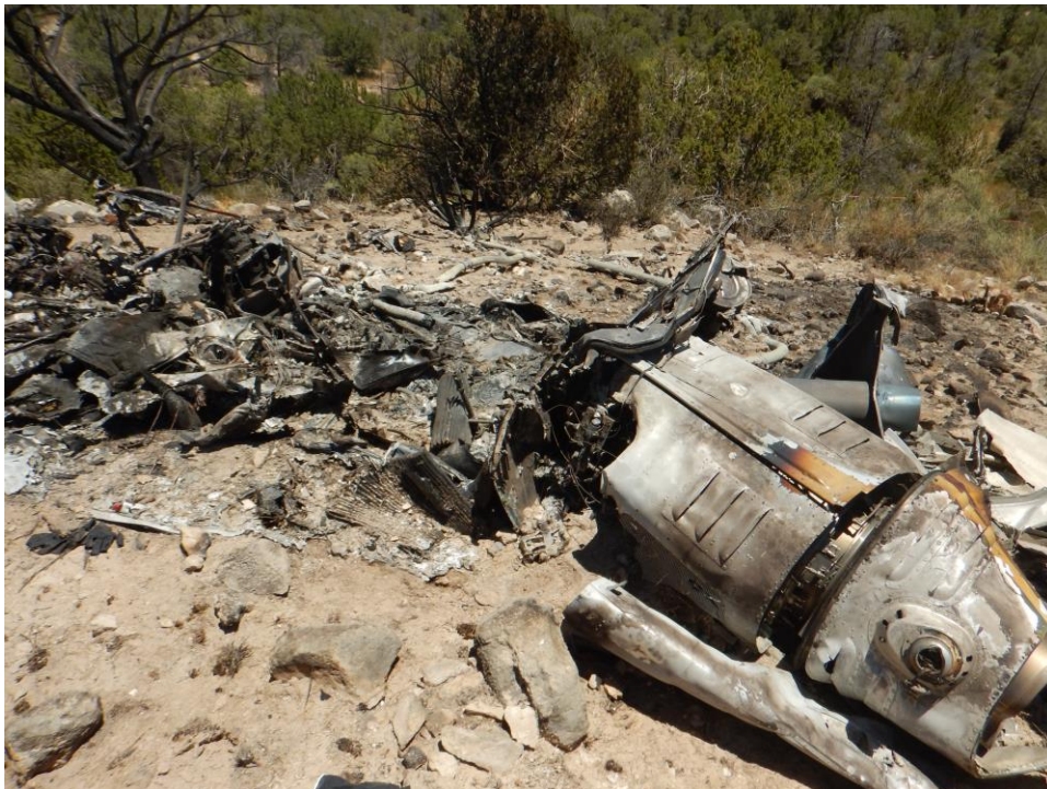
Figure 30. Engine Displaced and Separated from Mounts
