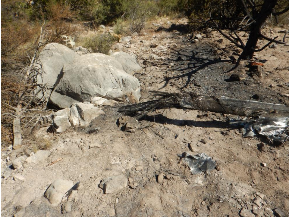
Figure 13. Broomstrawed Tip of Blade B
