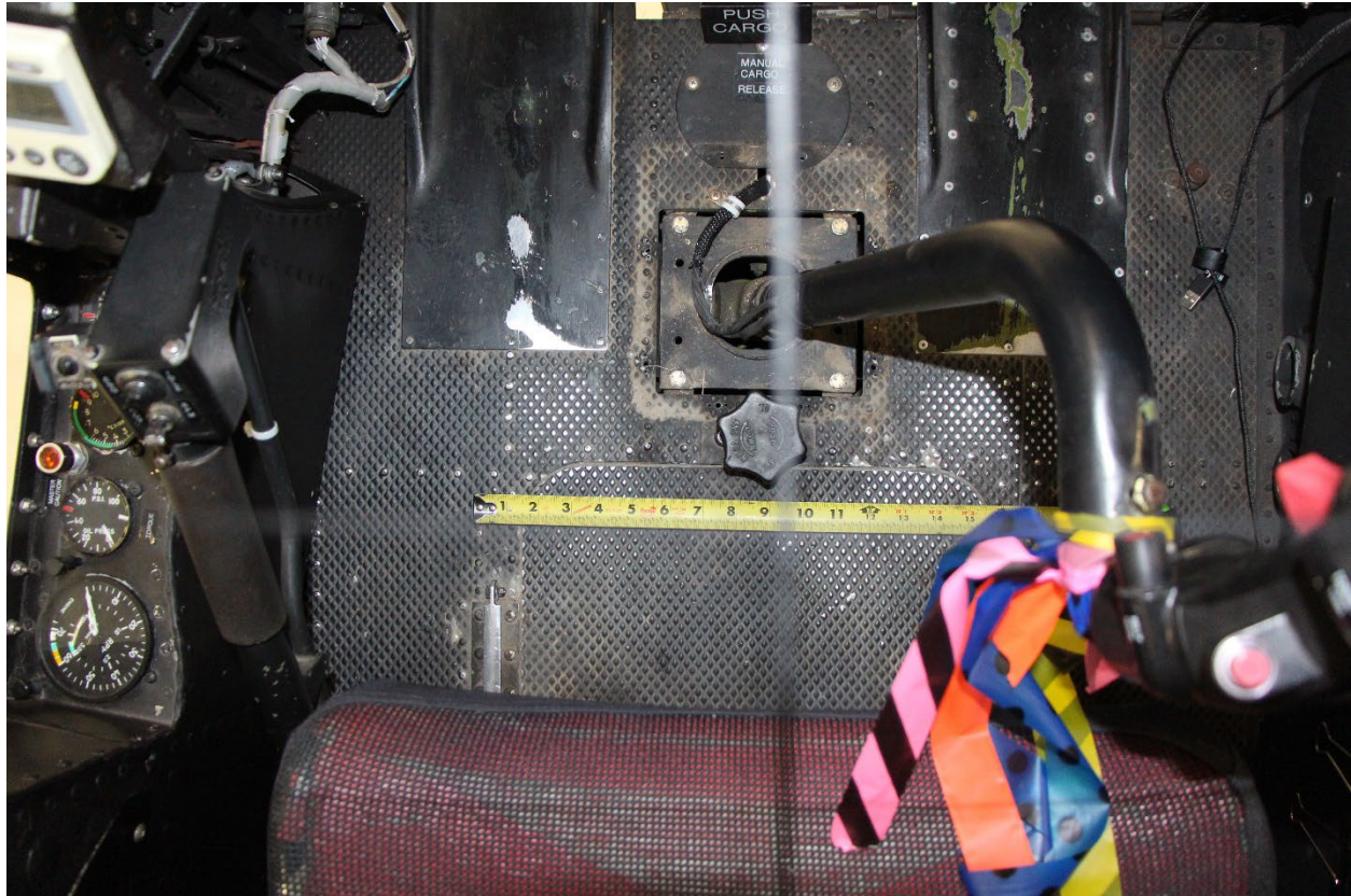
Photograph 2: Cyclic position of exemplar UH-1H when right servo shows 7 inches, left servo 9 inches
